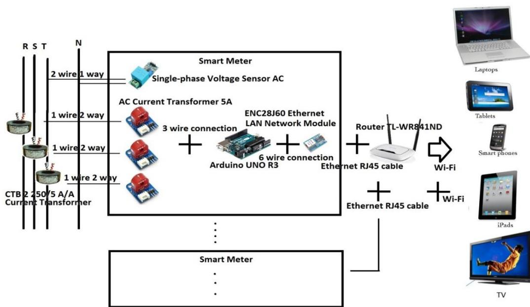
Figure 1. The architecture of the AMR system.
