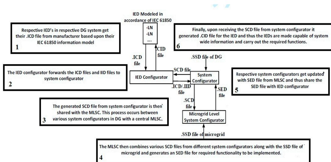
Figure 3. IEC 61850 microgrid communication configuration process.
