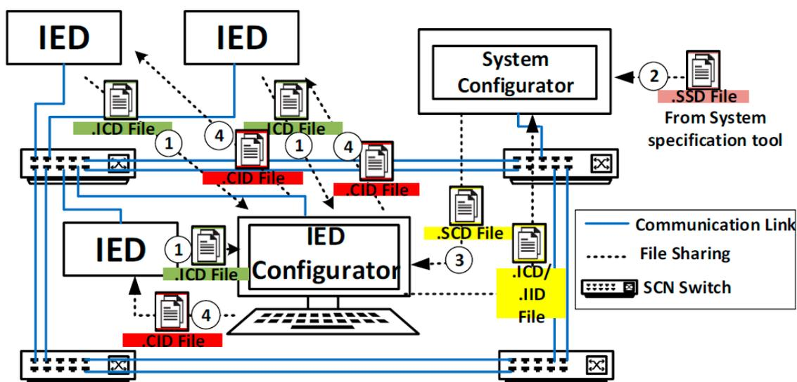
Figure 2. SCL file configuration for typical SCN.
