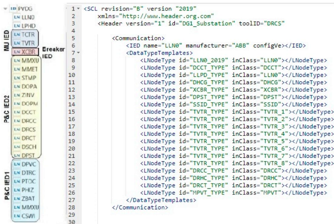
Figure 4. SCD file example for PV IED packed information.
