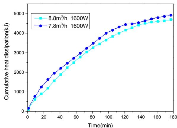
**Figure 13.** The heat dissipation of the system at different flow rates (the heat source power is 1600 W).
