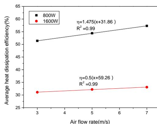
**Figure 8.** Correlation between average heat dissipation efficiency and air flow rate (cooling oil flow is 8.8 m<sup>3</sup>/h).
