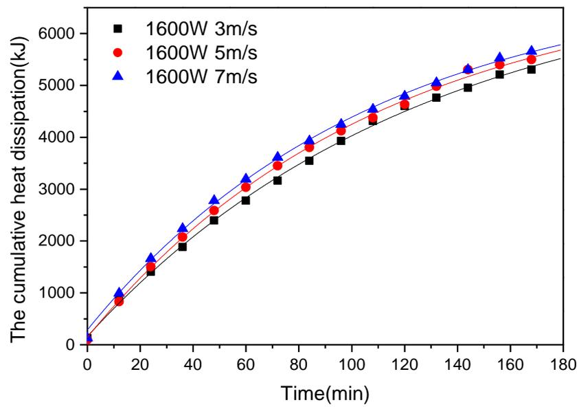
Figure 16. Test value logarithmic model regression fitting (cooling oil flow is 8.8 m<sup>3</sup>/h).
