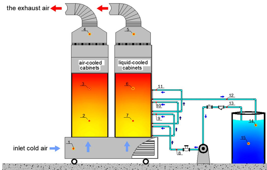
Figure 5. Image of the arrangement of all measuring points.
