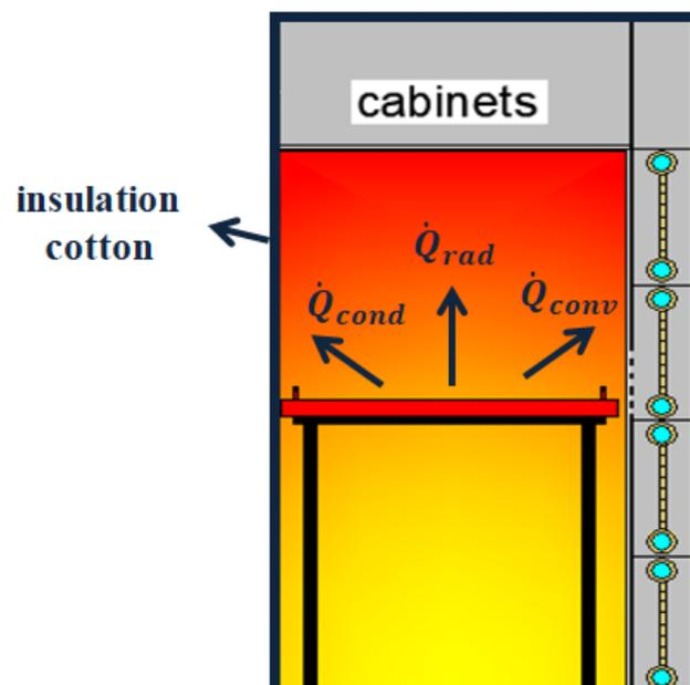
**Figure 6.** Schematic overview of the heat transfer balance for the cabinets.
