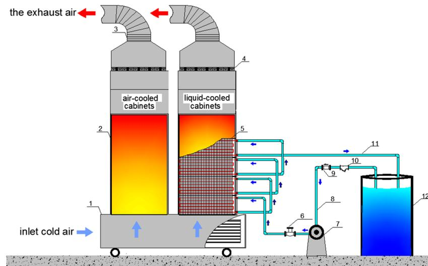
**Figure 1.** Schematic of the proposed system: 1—Movable downside air supply system; 2—Cabinet; 3—The top exhaust unit; 4—The top exhaust fan; 5—The rear door heat exchanger; 6—The flow valve; 7—The oil pump; 8—Oil pipeline; 9—The check valve; 10—The filter valve; 11—Oil return pipe; 12—The heat storage oil drum.
