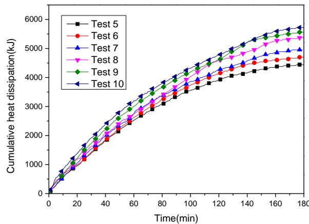
Figure 10. Trend of heat dissipation (cooling oil flow is 8.8 m<sup>3</sup>/h).
