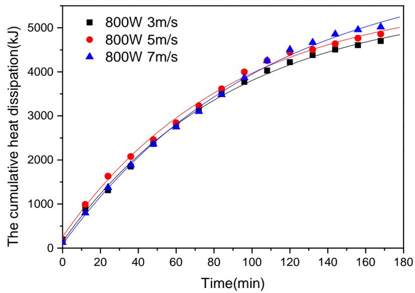
Figure 17. Test value logarithmic model regression fitting (cooling oil flow is 7.8 m<sup>3</sup>/h).
