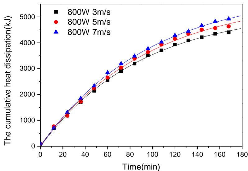
**Figure 15.** Test value logarithmic model regression fitting (cooling oil flow is 8.8 m<sup>3</sup>/h).
