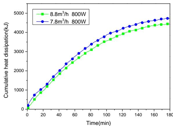
**Figure 12.** The heat dissipation of the system at different flow rates (the heat source power is 800 W).
