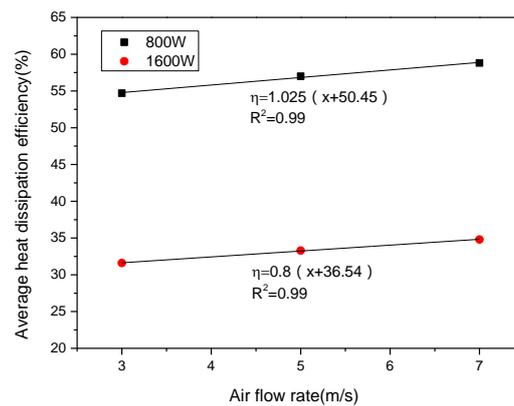
**Figure 9.** Correlation between average heat dissipation rate efficiency and air flow rate (cooling oil flow is 7.8 m<sup>3</sup>/h).
