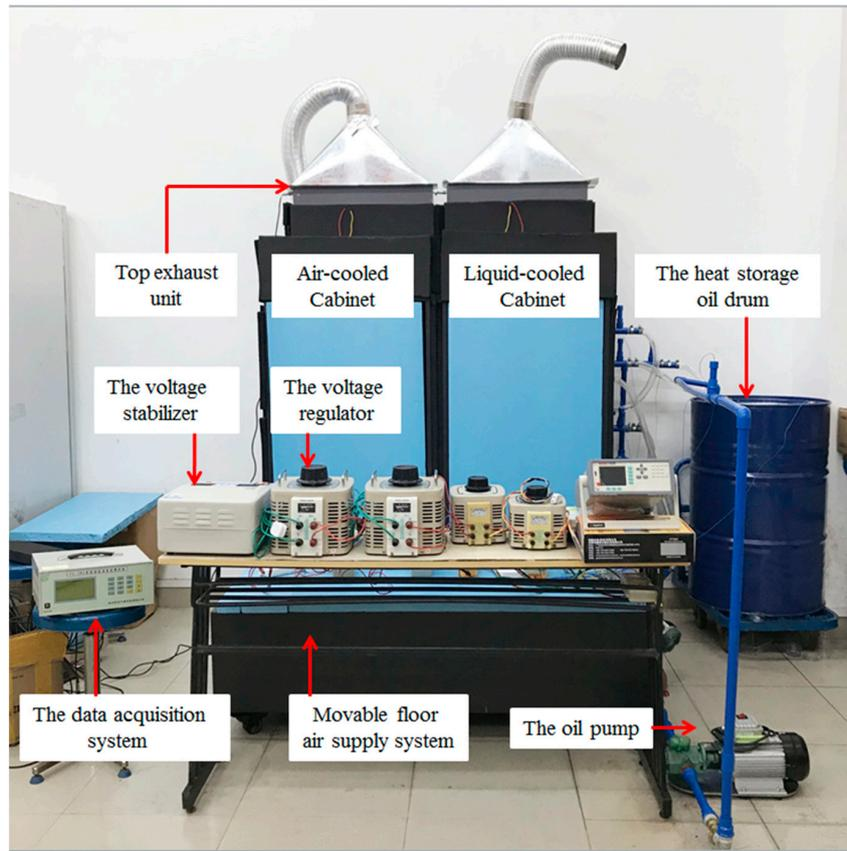
Figure 3. Image of the testing rig.
