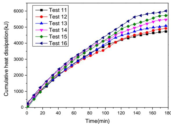
Figure 11. Trend of heat dissipation (cooling oil flow is 7.8 m<sup>3</sup>/h).
