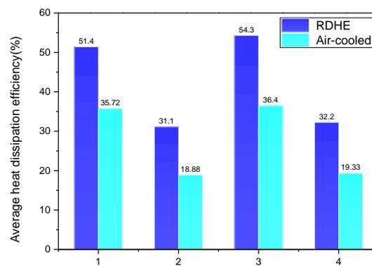
Figure 7. Comparison of air-cooled cabinets and liquid-cooled cabinets.
