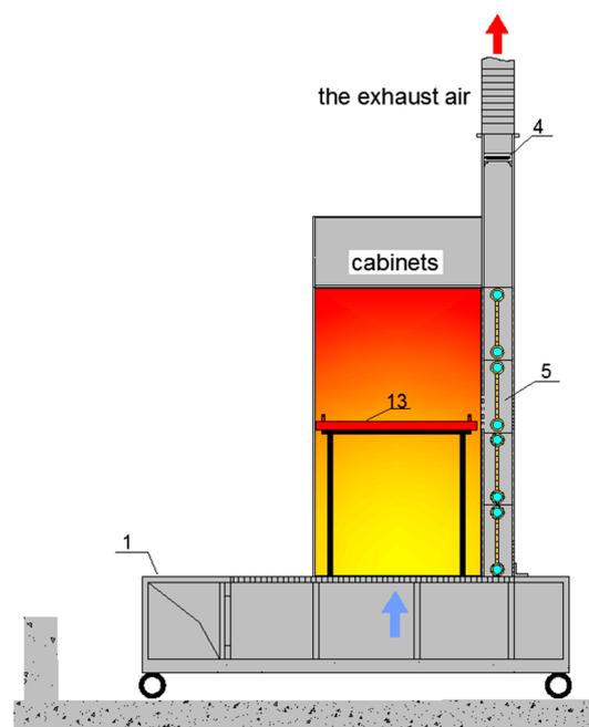
**Figure 2.** Schematic of the proposed system: 1—Movable downside air supply system; 4—The top exhaust fan; 5—The rear door heat exchanger; 13—The built-in analog heat source.
