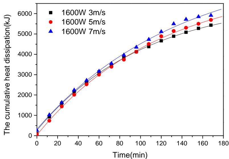
Figure 18. Test value logarithmic model regression fitting (cooling oil flow is  $7.8 \text{ m}^3/\text{h}$ ).
