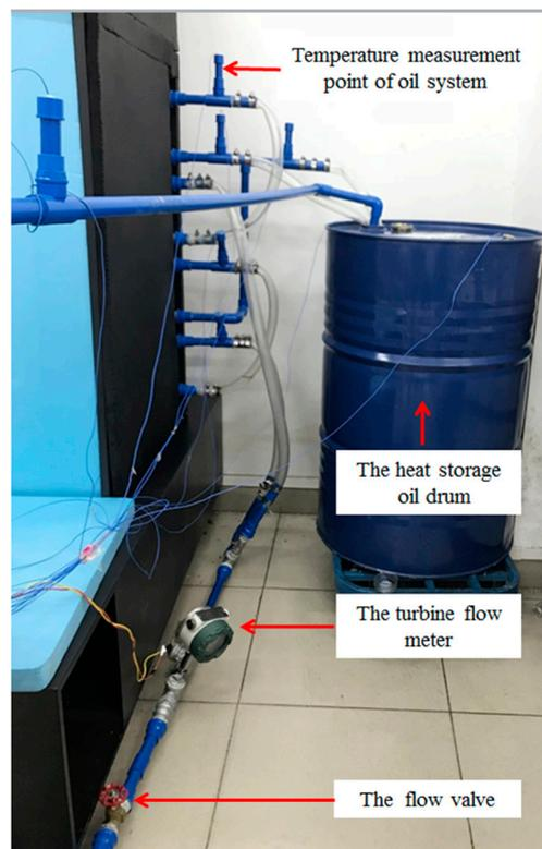
Figure 4. Image of the oil circuit system.
