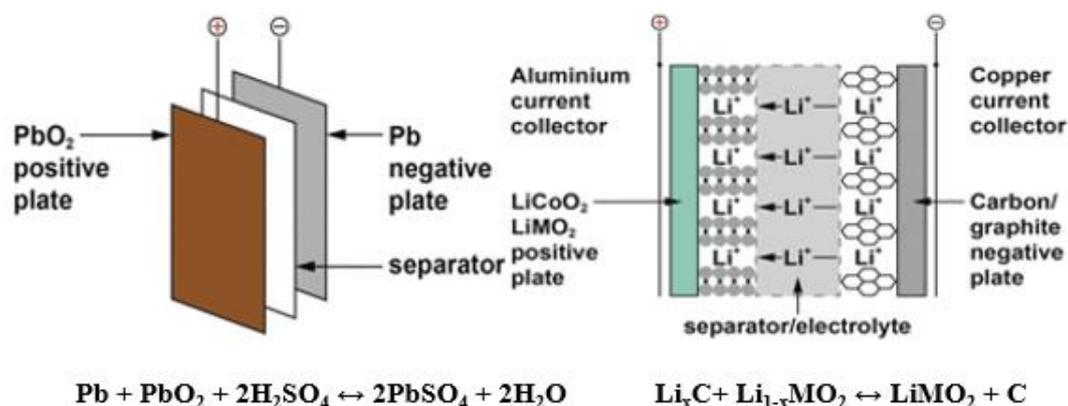
Figure 1. Principal components of lead–acid (left) and Li-ion (right) batteries [6].
