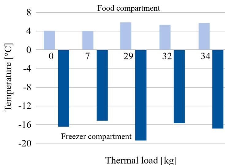
Figure 3. Thermal behavior of the compartments at 20 °C.
