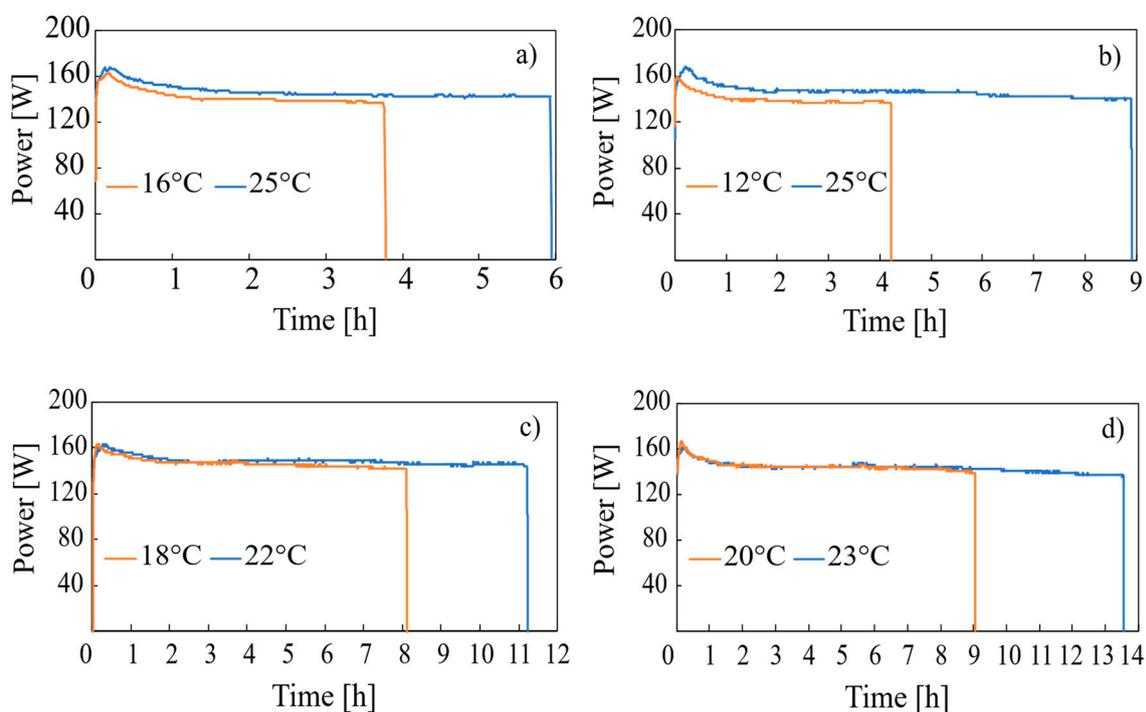
**Figure 11.** Consumed power in the start of the compressor for different thermal loads: (a) 13 kg; (b) 20 kg; (c) 23 kg; (d) 30 kg.
