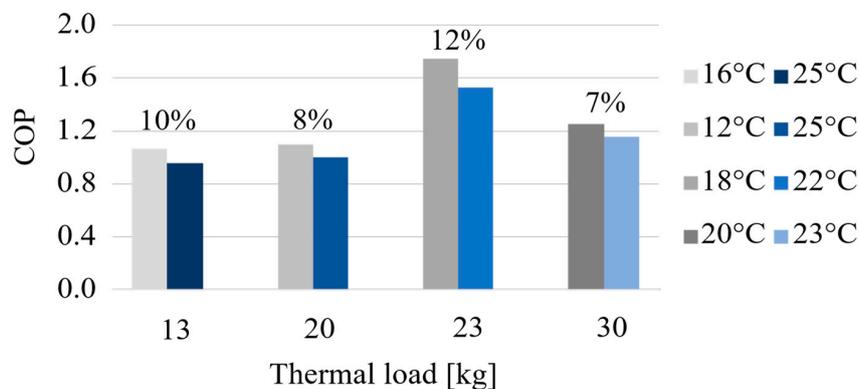
Figure 10. Coefficient of performance at different conditions of ambient temperature.
