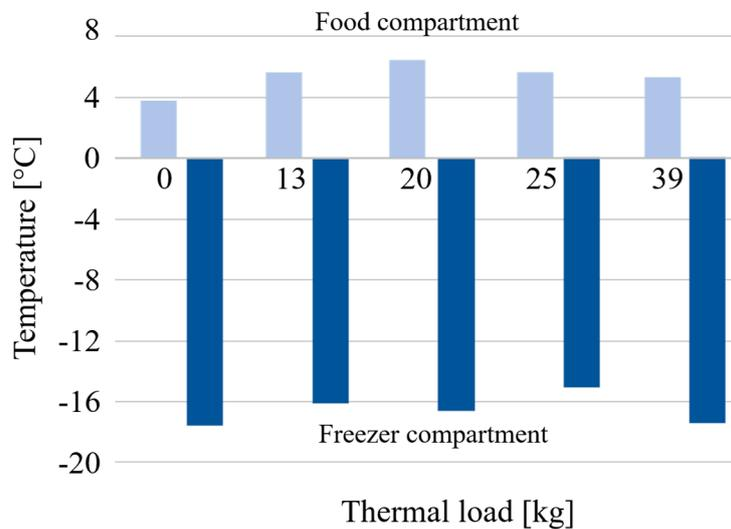
**Figure 4.** Thermal behavior of the compartments at 25 °C.
