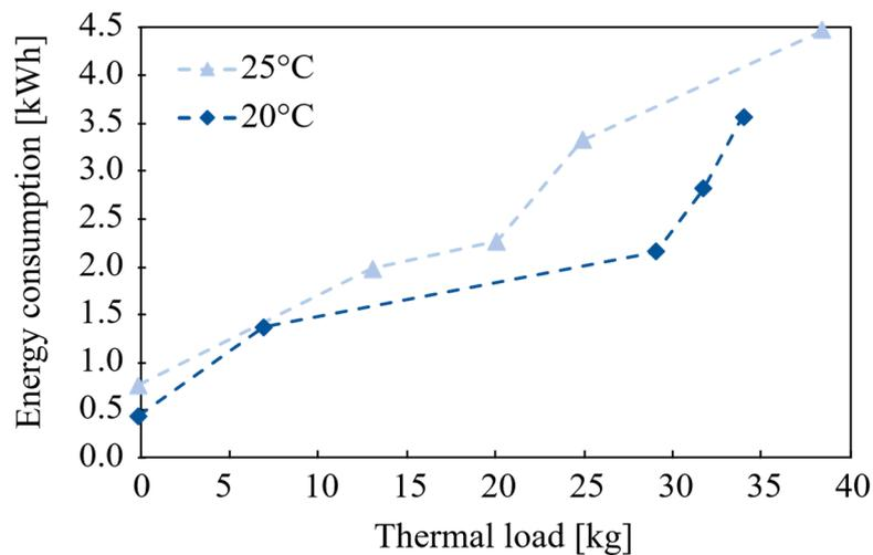
Figure 5. Energy consumption for different thermal loads.
