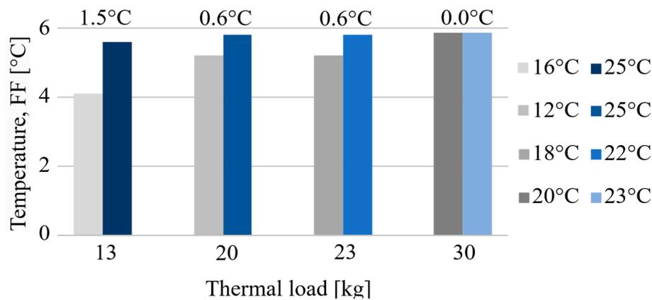
**Figure 7.** Temperature in the fresh-food compartment maintaining the constant thermal load at two ambient temperature conditions.
