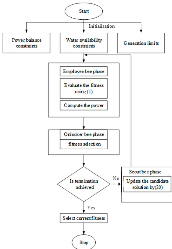
Figure 1. Flow chart of STHTS using proposed methodology.
