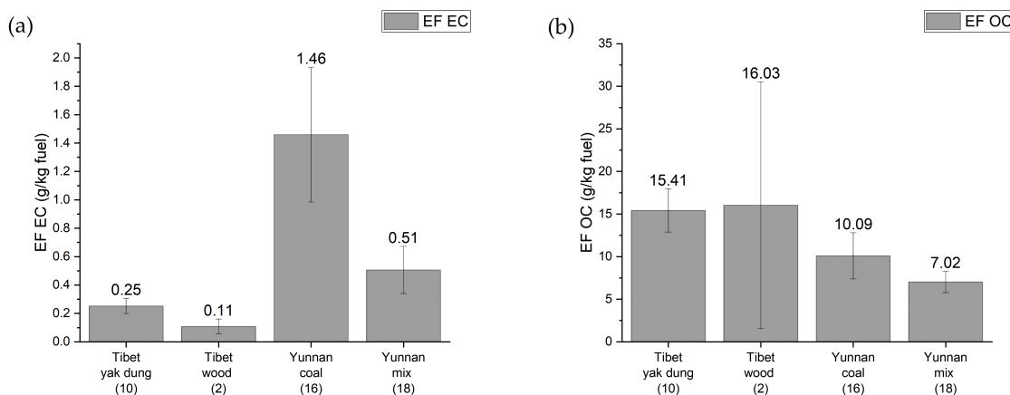
**Figure 10.** Comparison of carbon particulate emission factor between sites and fuels: (a) Elemental carbon; (b) Organic carbon.
