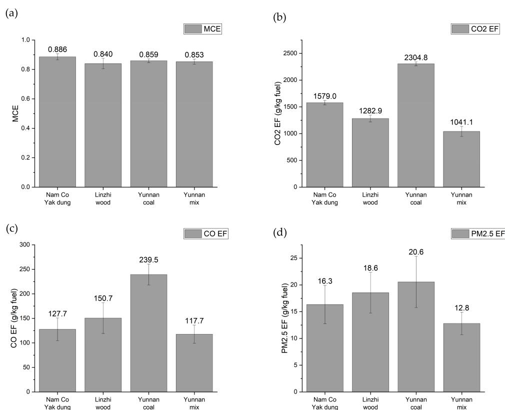
**Figure 9.** Comparison of emission parameters between sites and fuels: (a) Modified combustion efficiency (MCE); (b) Emission factor for  $\text{CO}_2$ ; (c) Emission factor for  $\text{CO}$ ; (d) Emission factor for  $\text{PM}_{2.5}$ .
