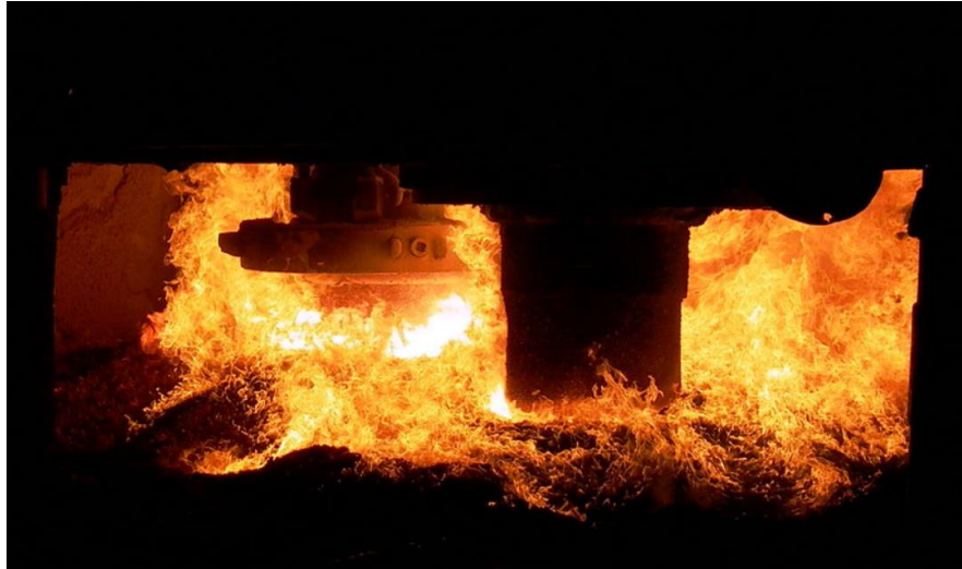
Figure 5. Picture of the upper part (zone 5, Figure 6) of a submerged ARC electrode furnace during process showing two electrodes in the center of the picture.
