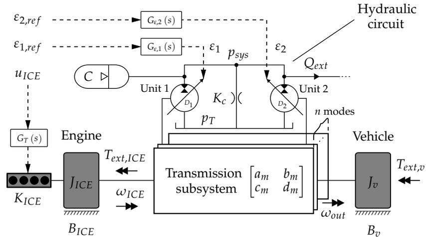
**Figure 1.** Linear lumped-parameter model of a general complex multi-mode hydraulic hybrid transmission with  $n$  modes, in mode  $m$ .  $Q_{ext}$  and  $T_{ext,ICE}$  are disturbances caused by, for instance, work functions, while  $T_{ext,v}$  is a disturbance from a load, e.g., a gravel pile.
