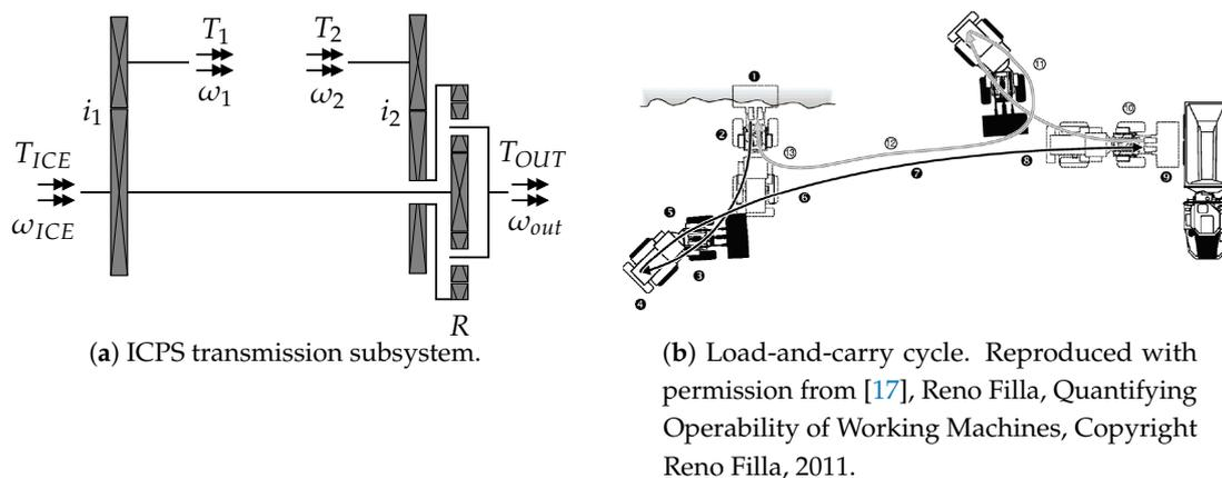
**Figure 4.** Reference vehicle transmission and drive cycle.
