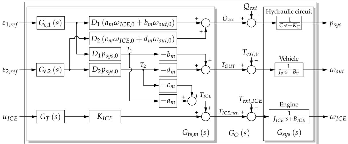
**Figure 2.** Block diagram of the linear model in Figure 1 at mode  $m$ , linearized at  $(p_{sys,0}, \omega_{out,0}, \omega_{ICE,0})$ .
