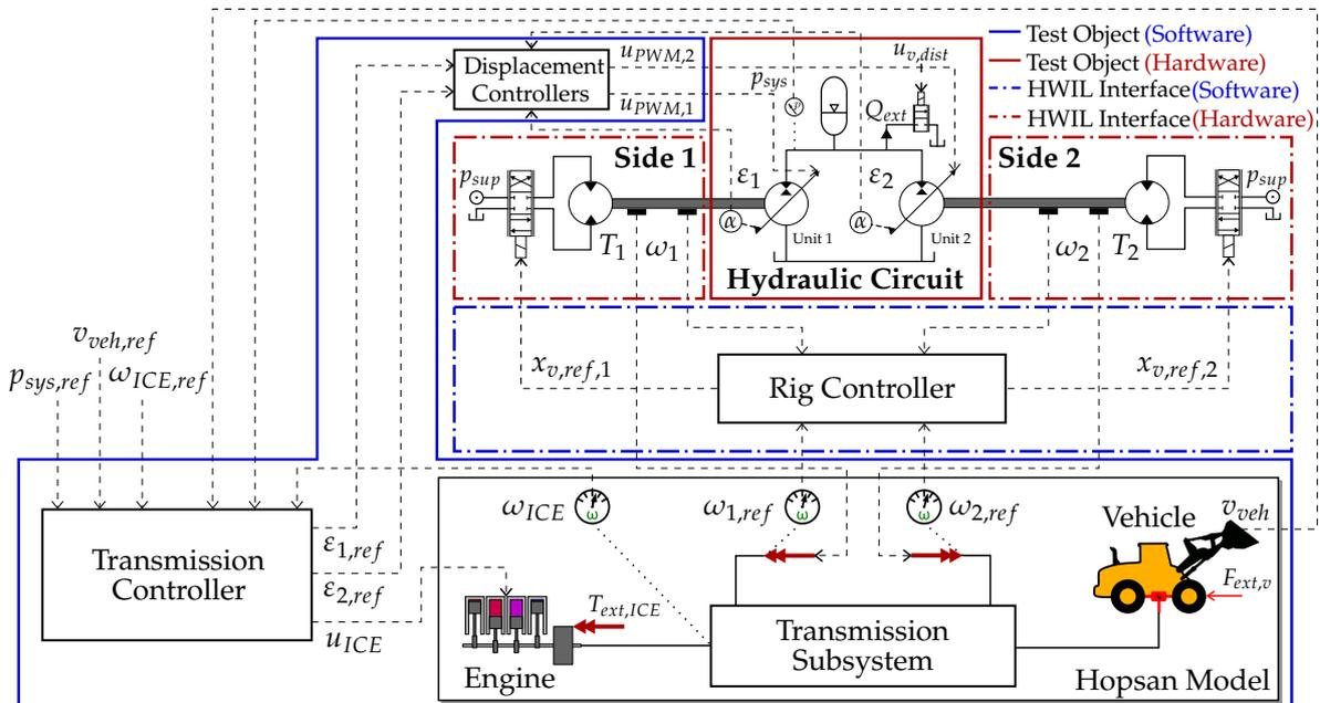
(b) Operation principle. Note that the vehicle is represented in the linear domain ( $\frac{\omega_{out}}{v_{veh}} = \frac{F_{ext,v}}{T_{ext,v}} = \frac{1}{l_0 r_w}$ ).
