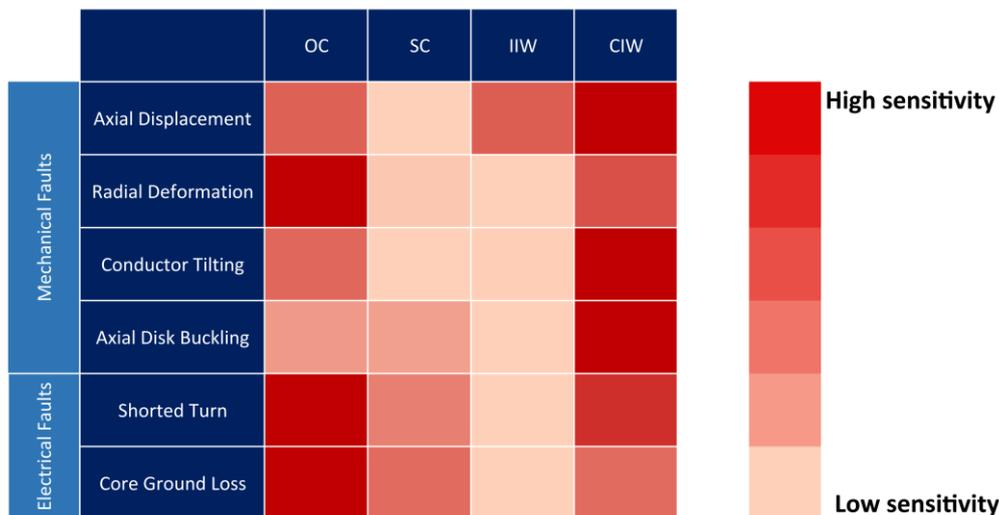
Figure 28. Identification of the most sensitive connection scheme for various electrical and mechanical faults; patterns are based on the minimum value of SDD (MSDD).
