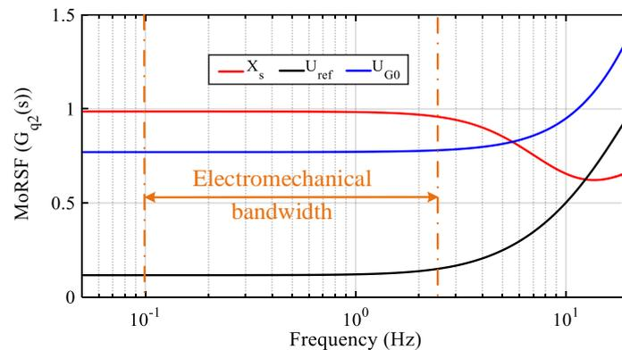
**Figure 7.** The magnitude of the relative sensitivity function (MoRSF) of  $G_{q2}(s)$  with respect to operation parameters.
