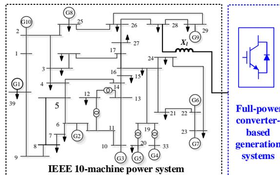
Figure 9. Single-line diagram of the (IEEE) 10-machine power system.
