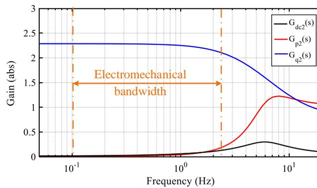
Figure 4. Bode gain diagram of the transfer function matrix.
