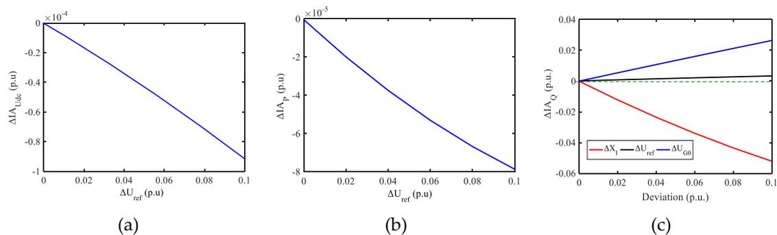
**Figure 13.** Initial amplitude( IA )deviation curves of (a) GVSC DC voltage, (b) active power, and (c) reactive power.
