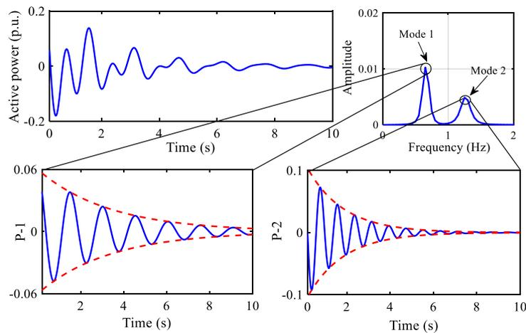
Figure 10. Time domain trajectory of active power from bus 28 to 29.
