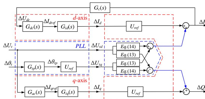
Figure 2. Small signal model of the GVSC.
