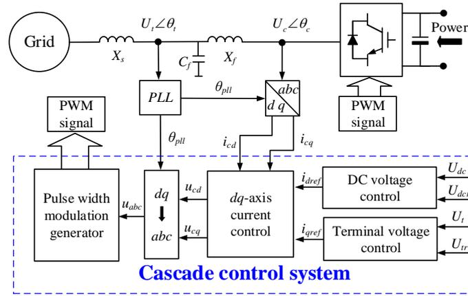
**Figure 1.** Topology and control system of grid-tied voltage source converter (GVSC).
