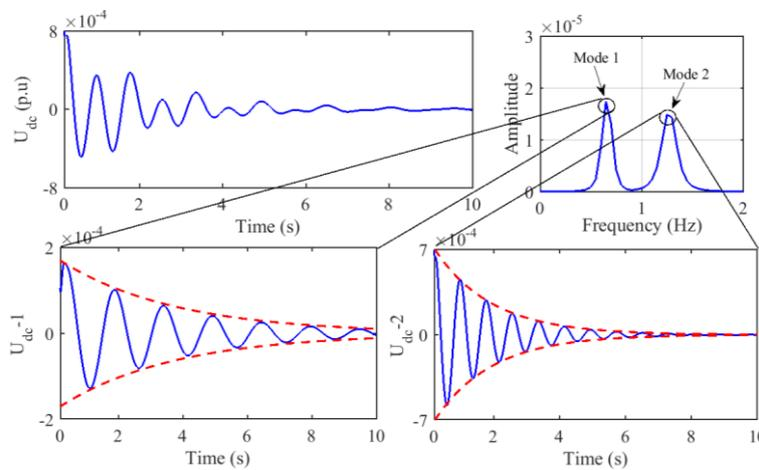
**Figure 11.** Time domain trajectory of DC voltage of GVSC.
