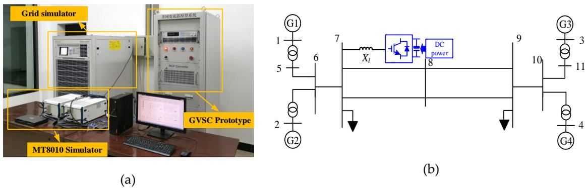
**Figure 14.** (a) Power hardware-in-the-loop (PHIL) platform. (b) Single line diagram of a two-area power system.
