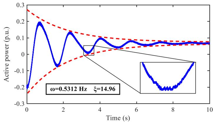
**Figure 15.** The measured response of tie-line active power.
