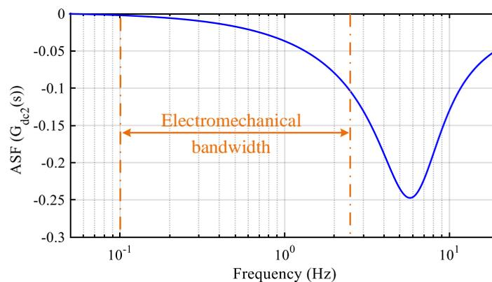
Figure 5. Amplitude sensitivity function (ASF) of  $G_{dc2}(s)$  with respect to  $U_{ref}$ .
