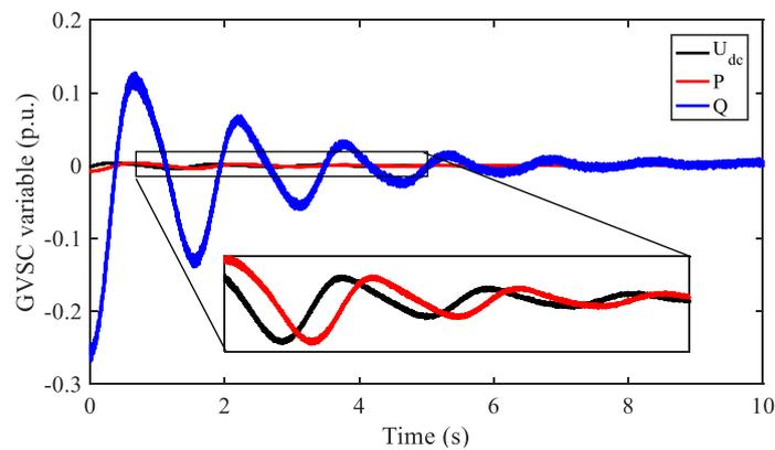
**Figure 16.** Measured response of port variables of GVSC.
