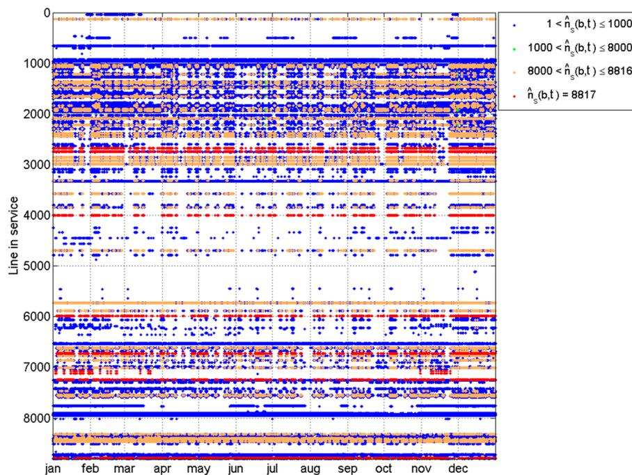
Figure 5. N–1 overloads for each line in each hour of yearly operation.
