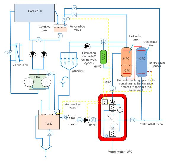
Figure 1. Operation of the heat recovery installation.
