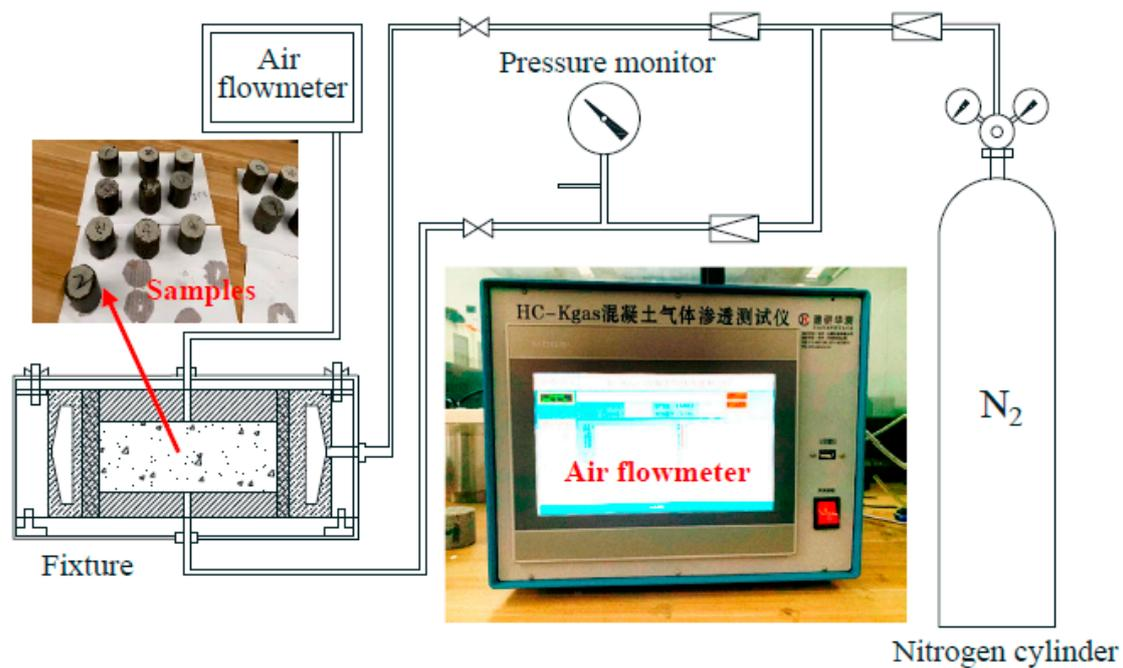
Figure 3. Gas permeability measurement system.
