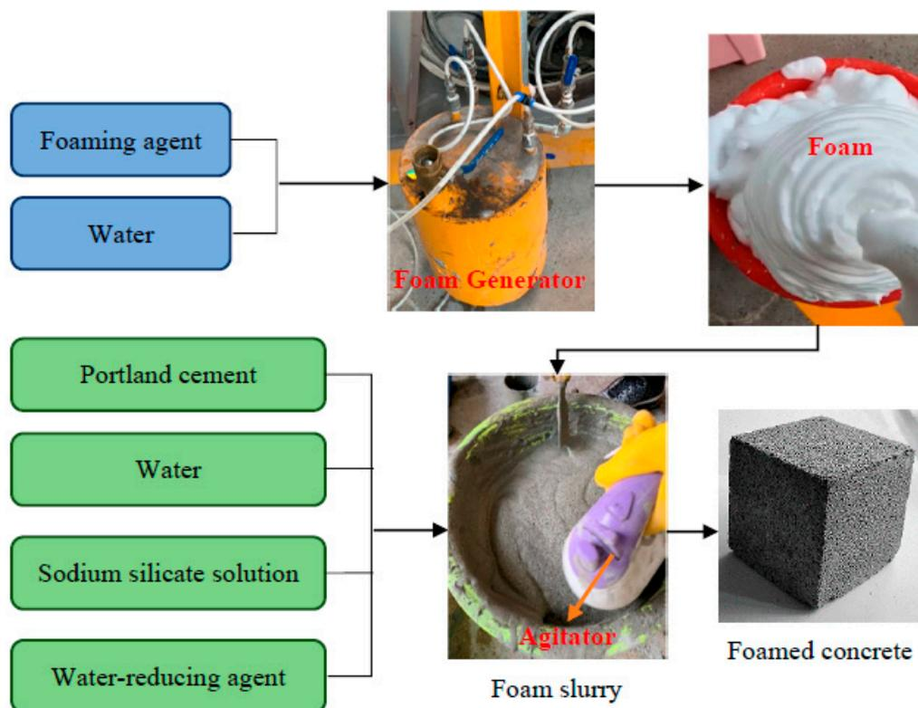
**Figure 1.** Procedure of specimen preparation.
