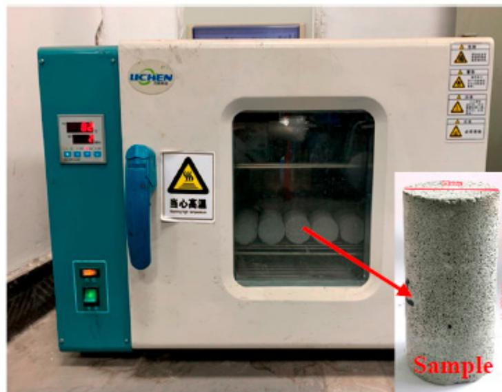
Figure 2. Constant temperature vacuum drying oven.
