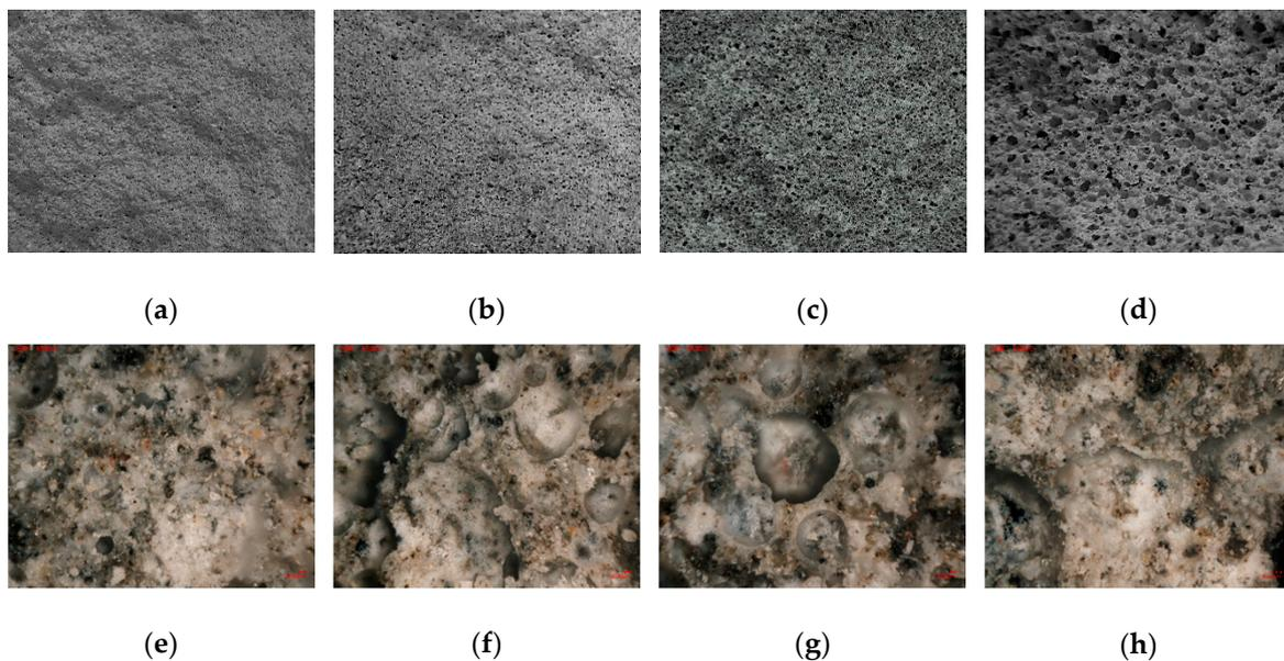
**Figure 6.** Pore structures of different foam content in 1 kg mass of solid powder: (a) 0.5 L foam; (b) 1.0 L foam; (c) 1.5 L foam; (d) 2.0 L foam; (e) 0.5 L foam ( $\times 500$  times); (f) 1.0 L foam ( $\times 500$  times); (g) 1.5 L foam ( $\times 500$  times); (h) 2.0 L foam ( $\times 500$  times).
