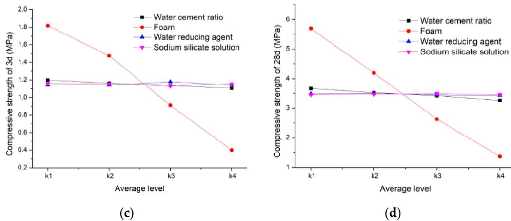
**Figure 5.** Average level of indicators under different factors: (a) average level of dry density; (b) average level of gas permeability; (c) average level of compressive strength of the 3rd day foamed concrete; (d) average level of compressive strength of the 28th day foamed concrete.
