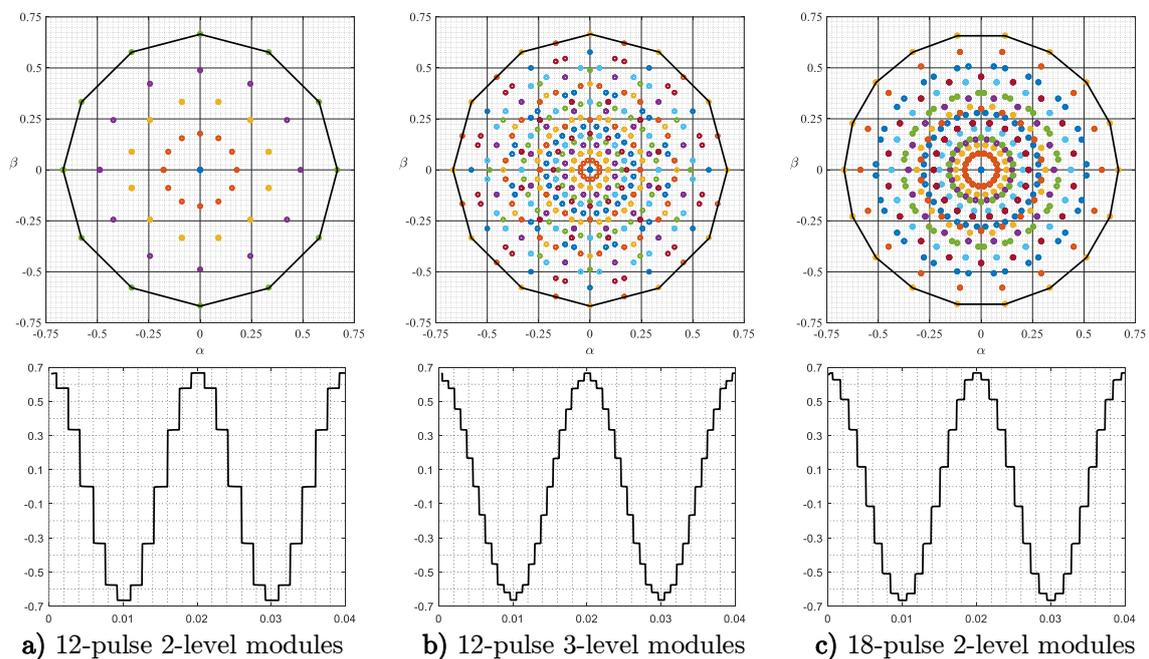
**Figure 5.** Space-vector diagrams of three modular VSI topologies (top graphs) and example voltage waveforms (bottom graphs) corresponding to the sequences of vectors indicated by connecting lines: (a) 12-pulse 2-level modules; (b) 12-pulse 3-level modules; (c) 18-pulse 2-level modules.
