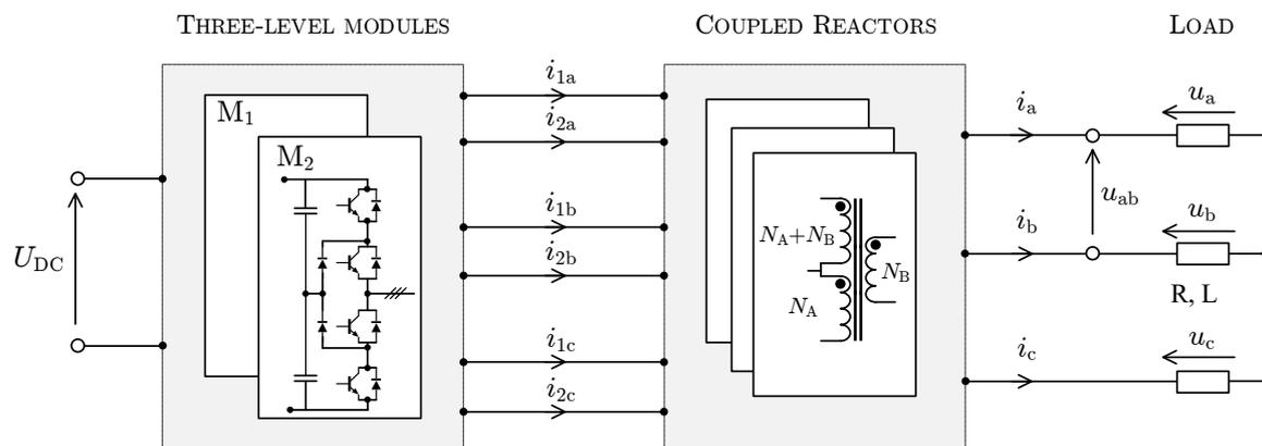
Figure 8. Twelve-pulse modular VSI with coupled reactors and three-level modules.
