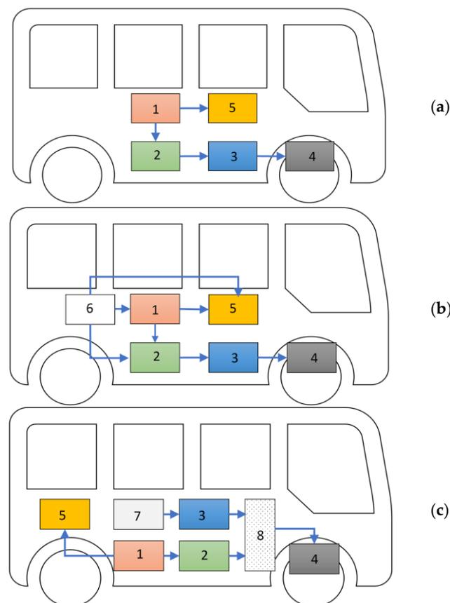
**Figure 1.** General structures of electric and hybrid powertrains used in the construction of buses: (a) electric bus; (b) hybrid series; and (c) hybrid parallel. 1, battery; 2, electric motor; 3, transmission; 4, final drive; 5, auxiliaries; 6, generator; 7, engine; and 8, torque converter/coupler.
