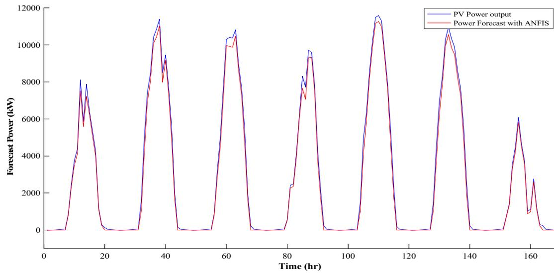
Figure 17. Weekly PV power output with ANFIS forecasting.
