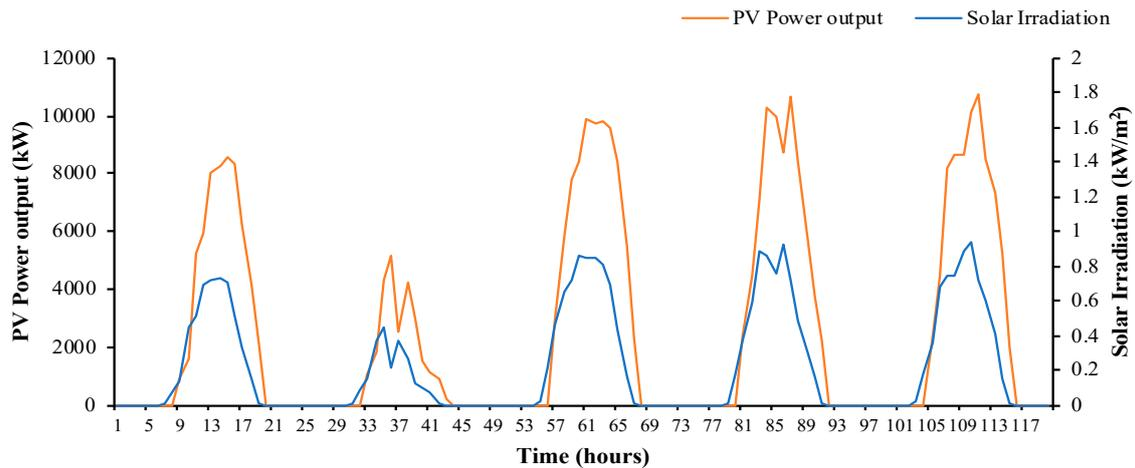
Figure 10. PV power output and solar irradiance.
