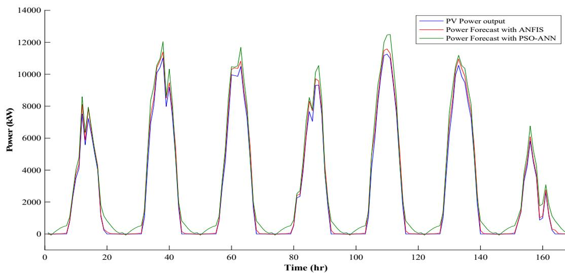
Figure 19. Comparison of PV power output forecasting.
