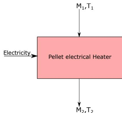
**Figure 3.** Mass and energy flows through the pellet heating unit.
