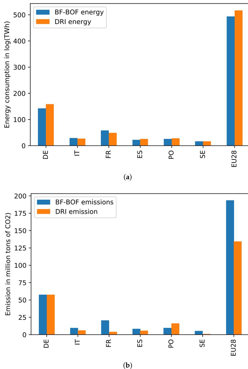
**Figure 13.** (a) Comparison of present energy demand from primary steel production in EU countries and projected energy demand for conversion to hydrogen direct reduction of iron ore (HDRI)-EAF based steel production. (b) Comparison of present emissions from primary steel production in EU countries and projected emissions for complete conversion to HDRI-EAF based steel production.
