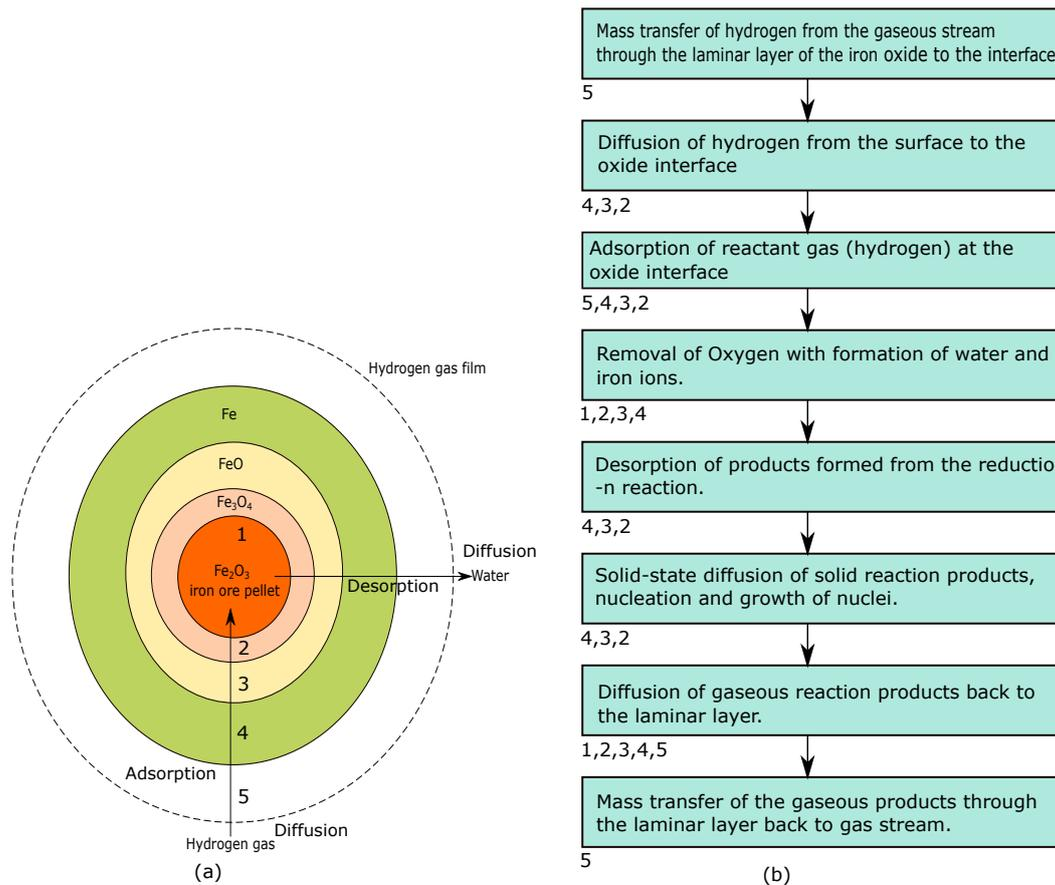
**Figure 1.** (a) Shrinking core model depicting the evolution of iron ore reduction reaction with hydrogen [56]. (b) Process steps in the reduction of iron ore pellets with hydrogen [37]. The location of the process steps is represented from numbers 1 to 5 (1b), which are also depicted in the shrinking core model (1a).
