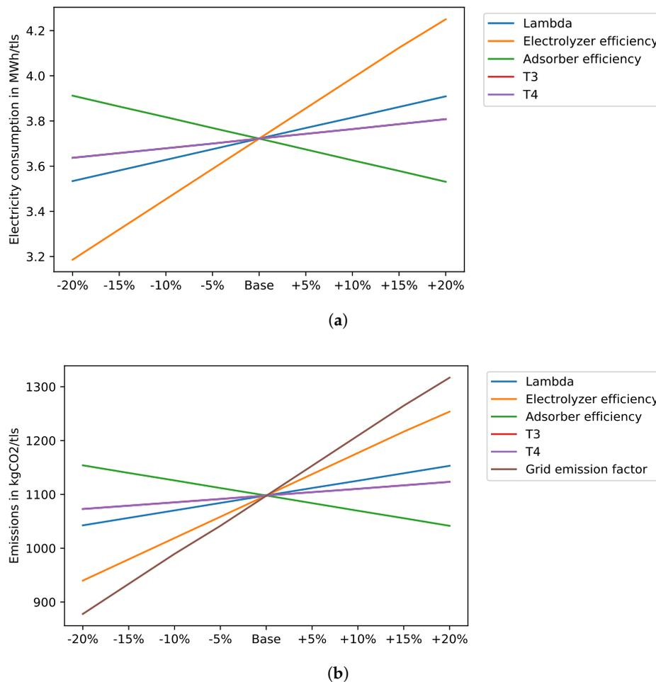
**Figure 14.** (a) Sensitivity analysis to identify the parameters affecting the electricity requirements of the HDRI-EAF system. (b) Sensitivity analysis to identify the most important parameters affecting the CO<sub>2</sub> emission from the HDRI-EAF system.
