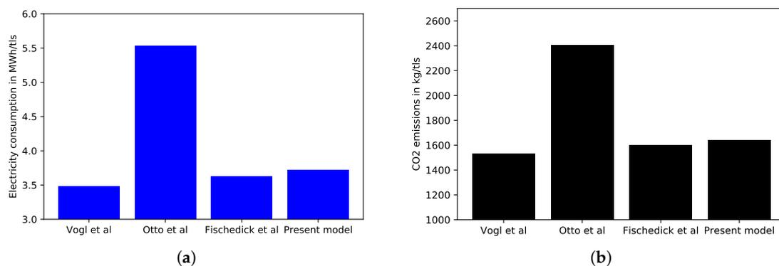
**Figure 12.** (a) Comparison of energy demand for hydrogen direct reduction of iron ore with literature values. (b) Comparison of CO<sub>2</sub> emission from hydrogen direct reduction of iron ore with literature values.
