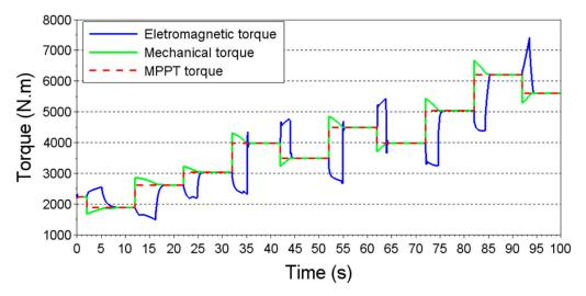
Figure 7. Difference between toques to accelerate the DFIG rotor.
