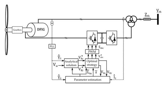
Figure 1. Proposed control and grid simulation topology.
