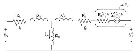
Figure 2. Equivalent circuit of the DFIG.
