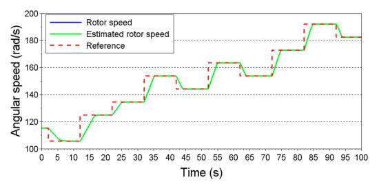
Figure 8. Estimation of rotor speed and its convergence to the reference value.
