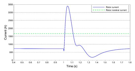
Figure 3. Rotor current after a reference step change compared to the rotor nominal current.
