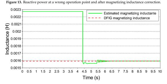
Figure 14. Correcting magnetizing inductance.
