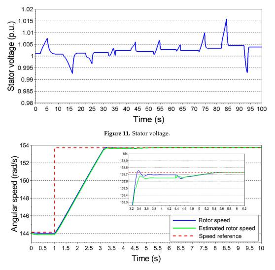
Figure 12. Estimated and actual rotor speed behavior of wrong and corrected magnetizing inductance values.
