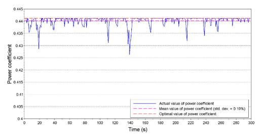
**Figure 19.** Comparison between the optimal value, the mean value and the actual value of the power coefficient.
