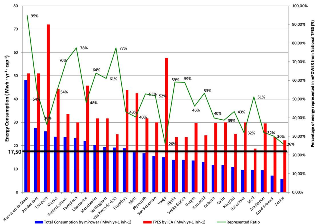
Figure 3. The total energy consumption by inhabitant computed for the selected cities (by mPOWER project) and the national reality reflected by the International Energy Agency averages. The goal in energy reduction of 17.5 MWh·cap<sup>-1</sup>·yr<sup>-1</sup> has been indicated [30].
