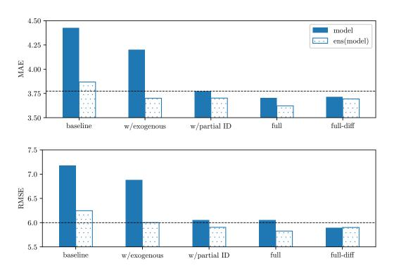
**Figure 4.** Bar plots illustrating the MAE (**top**) and RMSE (**bottom**) errors reported in the upper part of Table 1, that is, for the **naïve** benchmark and models that utilize back-transformation (4). The black dashed lines correspond to the benchmark, the solid bars represent the individual models and the dotted bars the corresponding ensembles.
