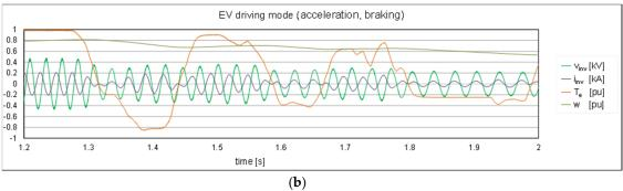
**Figure 4.** (a) EV driving state (accelerating and braking); (b) The zoom of the upper diagram, period (1.2–2) s.
