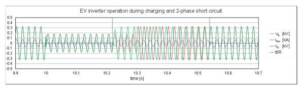
**Figure 7.** Inverter voltage and current and the network voltage during charging, 2-phase short circuit, island operation and again charging. The BR signal equal "0" means that BR breaker is closed.
