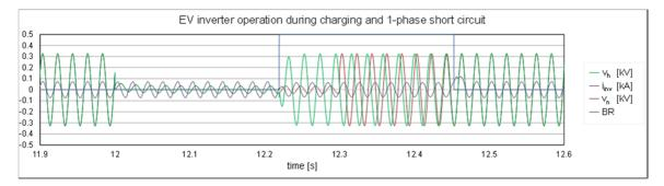
**Figure 8.** Inverter voltage and current and the network voltage during charging, 1-phase short circuit, island operation and again charging. The BR signal equal "0" means that BR breaker is closed.
