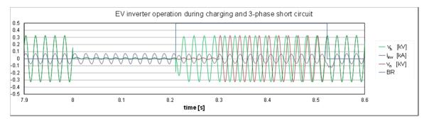
**Figure 6.** Inverter voltage and current and the network voltage during charging, 3-phase short circuit, island operation and again charging. The BR signal equeal "0" means that BR breaker is closed.
