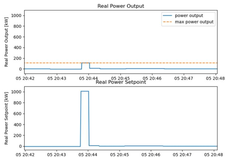
**Figure 3.** The real power output was set to 1010 kW, far above the 111.5 kW maximum power output.
