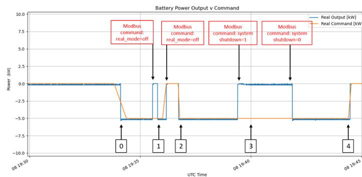
**Figure 2.** The real power outputs follow the Modbus commands even while being polled through the authenticated interface.
