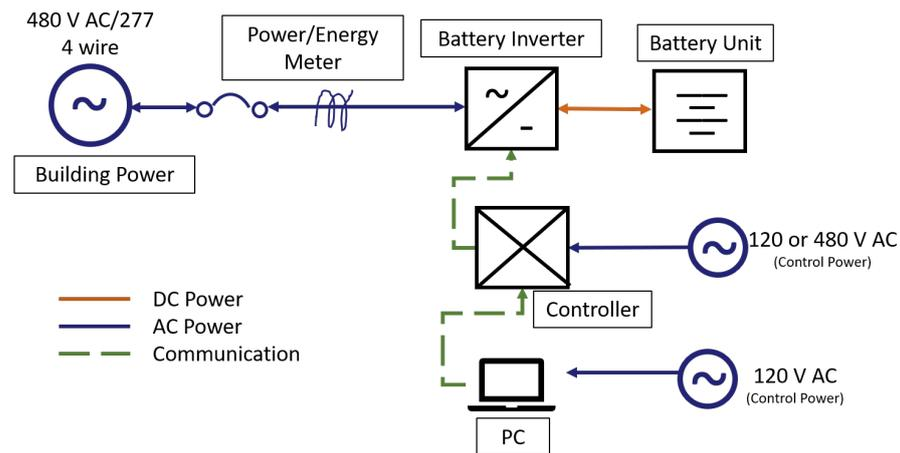
**Figure 1.** Hardware setup for grid-connected battery tests.
