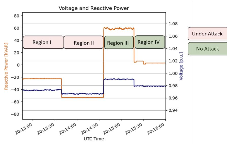
**Figure 4.** The adverse affects of a malicious Volt-VAR curve are shown in Regions I and II. Region III shows the effects from using a traditional Volt-VAR curve. Region IV shows the system voltage with no reactive power support.
