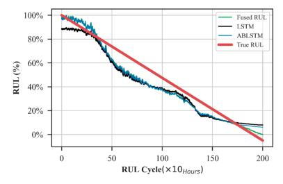
Figure 14. Prediction result of BiLSTM model on hybrid fault dataset.
