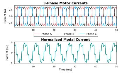
Figure 8. Modal current computation from the three-phase motor current.
