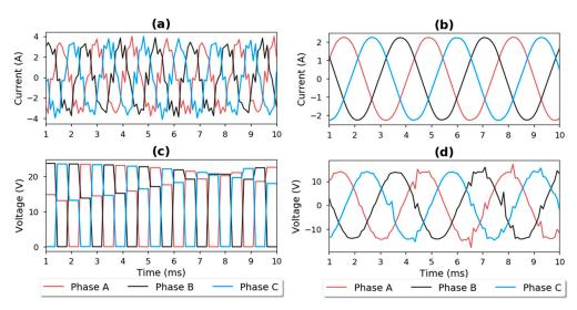
**Figure 7.** Sensor acquired current and voltage signals. (a) Motor current (input), (b) Generator current (output), (c) Motor voltage (input), (d) Generator voltage (output).
