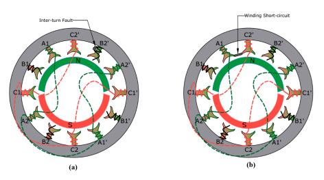
Figure 6. (a) Inter-turn short circuit fault. (b) Winding short-circuit fault.
