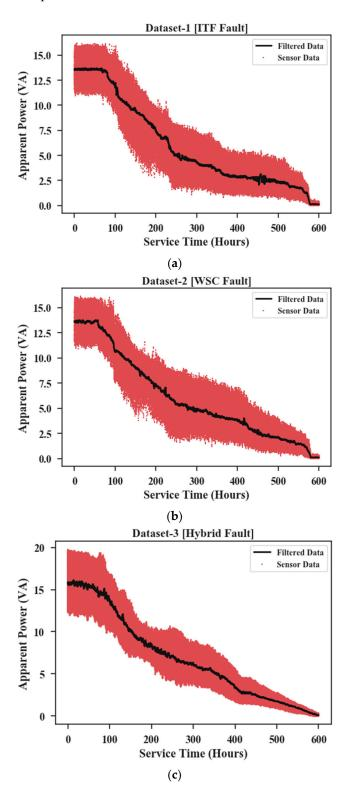
Figure 12. Degradation data of different fault states. (a) ITF fault, (b) WSC fault, (c) Hybrid fault.
