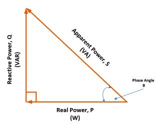
Figure 2. Power triangle of AC power system.
