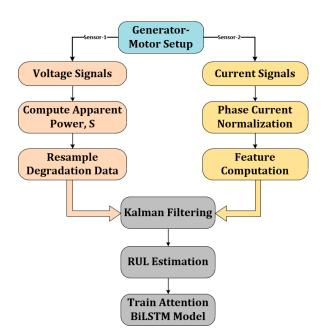
Figure 1. Graphical illustration of the proposed RUL estimation method.
