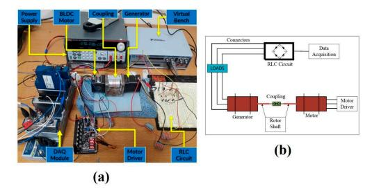
Figure 5. Test rig setup. (a) Reat test bench photo, (b) Schematic diagram of the test bench setup.
