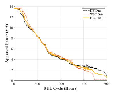
Figure 13. RUL estimation from ITF and WSC degradation data.
