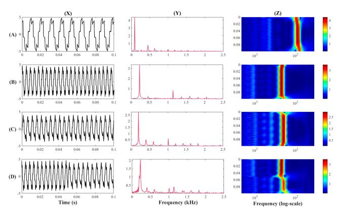
**Figure 9.** Third harmonic (H3) analysis of the motor currents in healthy state (row **A**), ITF fault state (row **B**), WSC fault state (row **C**), hybrid fault state (row **D**). Column X is the sensor acquired time series signal, column Y is the FFT transformation, column Z is the time-frequency representation using CWT.
