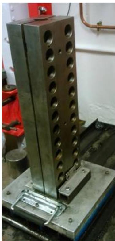
Figure 6. Hexagonal split mold.
