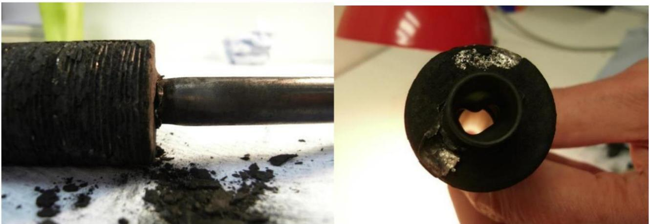
**Figure 4.** Preliminary trials with cylindrical modules caused crushing of the central tube.
