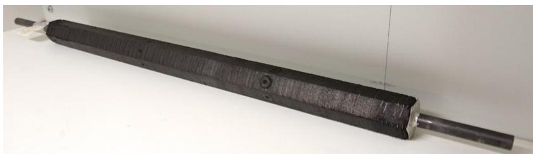
Figure 7. Completed aluminum-carbon laminate tube module.
