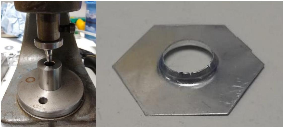
**Figure 5.** Fin collar forming swaging tool (left) and the resulting fin (right).
