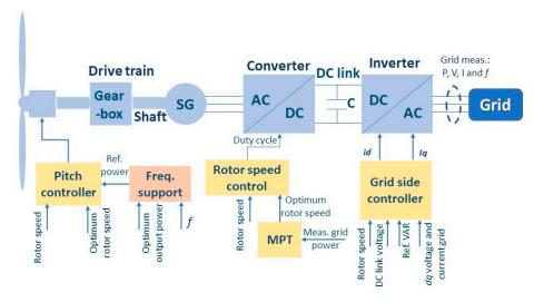
Figure 6. Schematic of the implemented Type 4 WTG and the associated controls.
