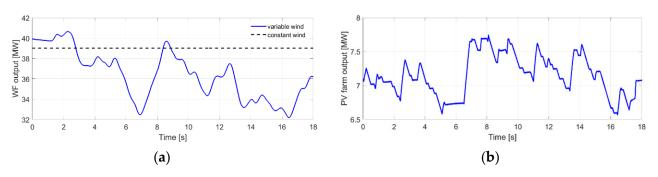
Figure 11. Output power: (a) wind farm under conventional operation; (b) PV farm under conventional operation.
