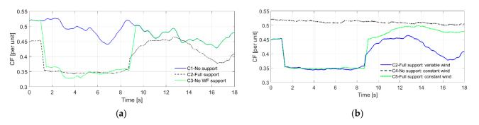
Figure 13. Capacity factor: (a) variable wind speed; (b) constant wind speed compared to Case 2.
