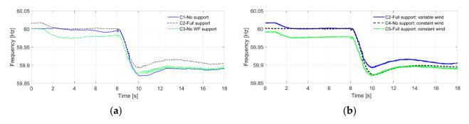
Figure 14. System frequency measured at the HPP point of connection: (a) variable wind speed; (b) constant wind speed compared to Case 2.
