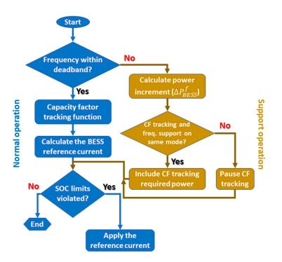
Figure 2. Flowchart of the proposed coordination between frequency support and CF tracking.
