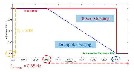
Figure 4. A<sub>F</sub> setting according to frequency variability and method of deloading.
