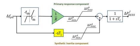
Figure 1. Frequency support controller of the BESS.
