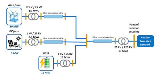
Figure 5. Single line diagram of the HPP and its connection to power network.
