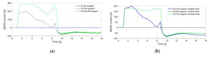
Figure 10. BESS cell current: (a) Variable wind speed; (b) Constant wind speed compared to Case 2.
