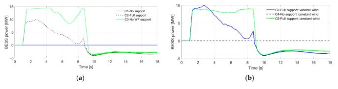
Figure 12. BESS total power: (a) variable wind speed; (b) constant wind speed compared to Case 2.
