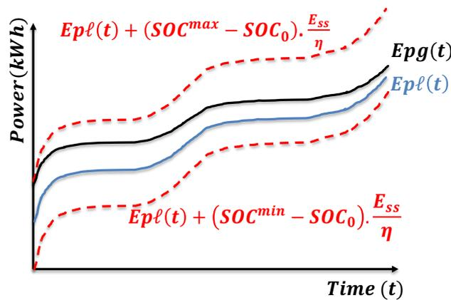
**Figure 3.** In order to keep SOC limitations,  $Epg$  must stay between two dotted lines determined by  $Epl + SOC_{min}$  and  $Epl + SOC_{max}$ .
