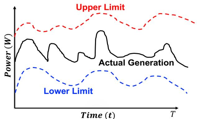
**Figure 12.** Power supply limitation based on historic data.
