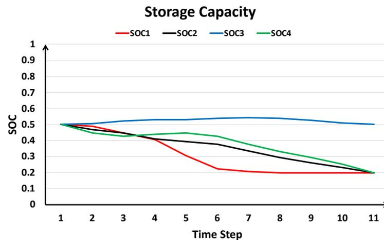
**Figure 15.** Change of SOC in time when power generators generate lower limits and power loads consume upper limits.
