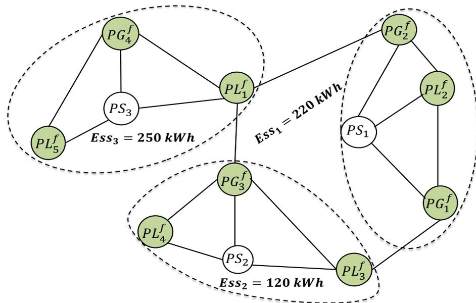
Figure 24. One possible localization for installing storage devices.
