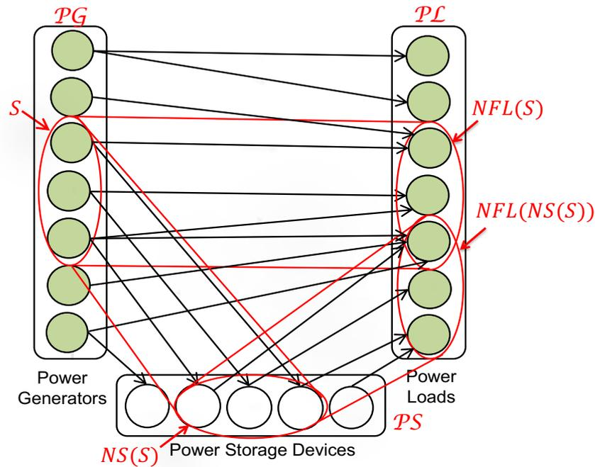
Figure 7. Subset  $S$  of power generators and the neighbor connected set of power devices.
