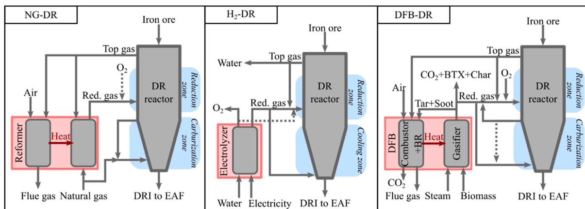
**Figure 2.** Schematic of the DR routes compared in this work. NG-DR refers to the traditional, natural-gas-based DR using the MIDREX technology, H<sub>2</sub>-DR refers to DR using hydrogen produced from electrolysis, and DFB-DR refers to the DR of iron using gas derived from DFB biomass gasification. The H<sub>2</sub>-DR and DFB-DR routes are based on a MIDREX DR reactor. *Red. gas* refers to the reducing gas, and *BR* refers to the bed reducer.
