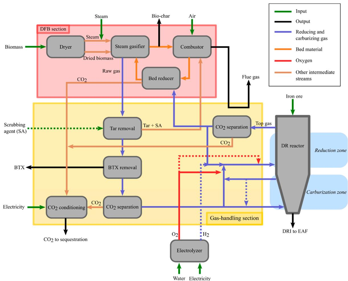
**Figure 3.** Schematic of the proposed DFB-DR route. The EAF section and downstream steel processing are not shown. Dashed lines indicate optional streams. The thicknesses of the arrows are not scaled to the sizes of the respective flows.
