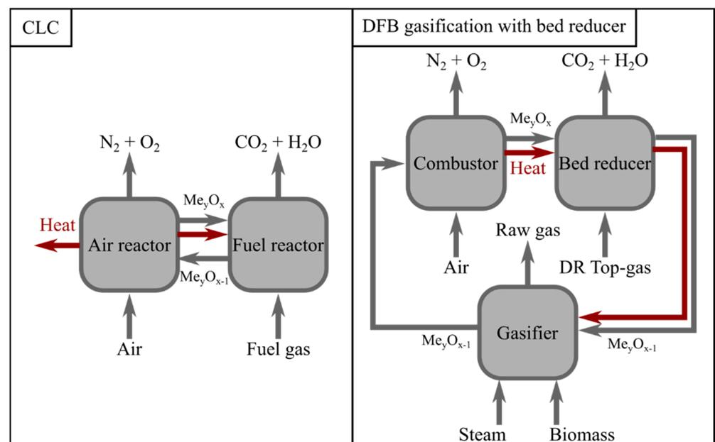
**Figure 1.** Schematic of the gas chemical-looping combustion technology (left-hand panel) and of the DFB gasification loop in the proposed process (right-hand panel), where a bed reducer section is introduced. Me<sub>y</sub>O<sub>x</sub> refers to the oxidized oxygen-carrying bed material, with Me referring to metal, and Me<sub>y</sub>O<sub>x-1</sub> is the reduced form of the oxygen carrier.
