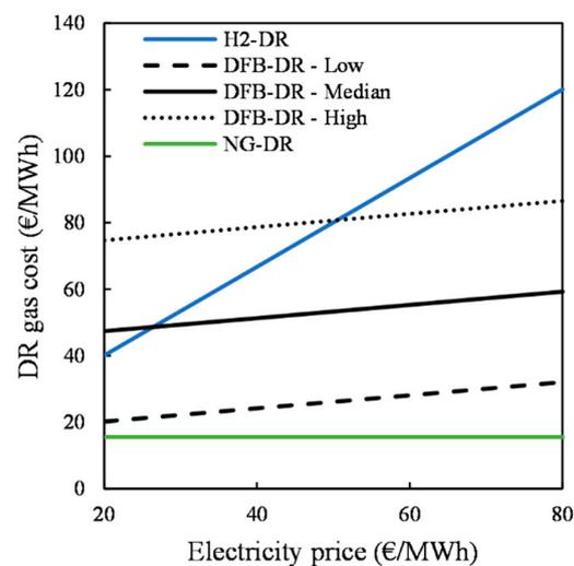
**Figure 6.** Costs for the reducing gas sent to the DR reactor for the three DR routes. For the DFB-DR route, the “Low” series is based on a biomass price of 0 EUR/MWh and the lower boundary of the CAPEX of the DFB loop and the gas-handling section, whereas the “High” series is based on a biomass price of 40 EUR/MWh and the upper boundary of the CAPEX.
