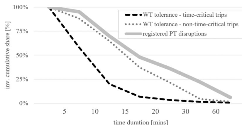
**Figure 6.** Results—revealed distribution of waiting time tolerance in the event of PT disruptions (acc. to surveyed passengers), plotted against the distribution of actual duration of PT suspension events (acc. to the PT operator's registry).
