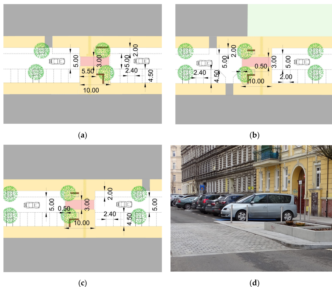
Figure 6. Treatments of chokers/raised pedestrian crossings: (a) testing ground No. 1; (b) testing ground No. 2; (c) testing ground No. 3; (d) design details of the sinusoidal approach ramp to the raised crossing and a view of a concrete planter. Source: own work of the author based on the design documentation [40].
