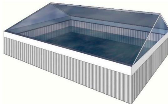
Figure 1. 3D schematics of a double-slope solar still.
