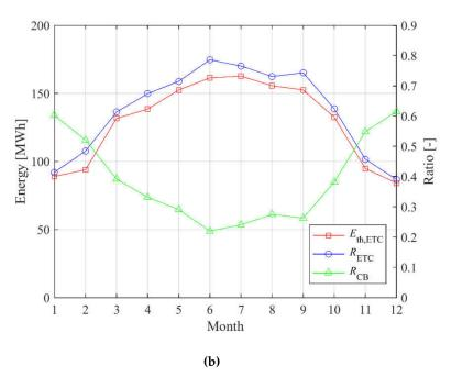
**Figure 10.** Monthly results: energy performance of the ETC of the PS3 for the scenario of **(a)** Naples and **(b)** Fayoum.
