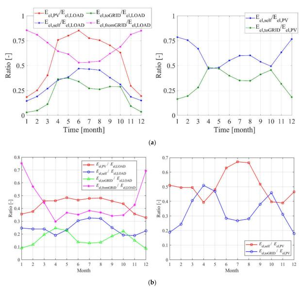
**Figure 9.** Monthly results of the energy ratios of the electric energy demand and energy ratios of the produced photovoltaic (PV) electric energy of the third proposed system (PS3) for the districts located in (a) Naples and (b) Fayoum.
