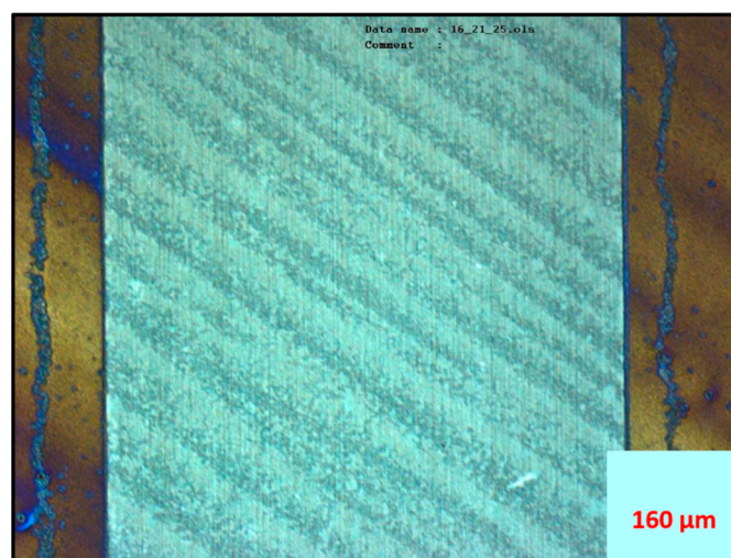
Figure 2. Ablated area obtained by 2-step P2 laser ablation over \text{mTiO}_2+\text{G}/\text{perovskite}/\text{PTAA} stack.
