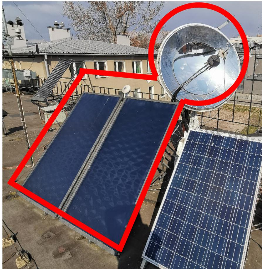
**Figure 1.** Parabolic dish concentrator with two focusing elements: bowl lined with reflective foil and parabolic mirror.
