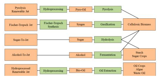
Figure 1. Raw materials used for the production of aviation biofuels and the corresponding processing [17].
