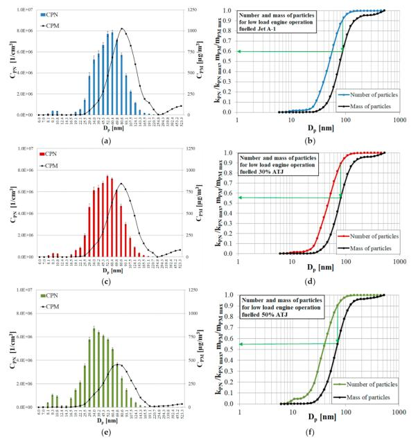
**Figure 5.** Number and mass concentration of particles depending on their diameter (a,c,e) and cumulative values of the relative particles number and relative mass of particulate matter (b,d,f) for low engine operation load fueled Jet A-1 (a,b), 30% ATJ (c,d) and 50% ATJ (e,f).
