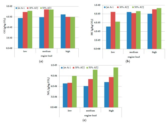
Figure 3. Emission index for (a) carbon monoxide; (b) hydrocarbons; (c) nitrogen oxides.
