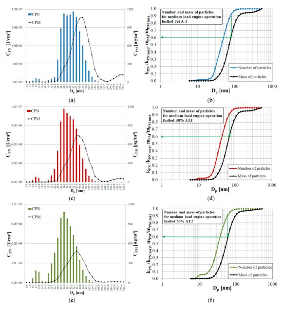
**Figure 6.** Number and mass concentration of particles depending on their diameter (**a**,**c**,**e**) and cumulative values of the relative particles number and relative mass of particulate matter (**b**,**d**,**f**) for medium engine operation load fueled Jet A-1 (**a**,**b**), 30% ATJ (**c**,**d**) and 50% ATJ (**e**,**f**).
