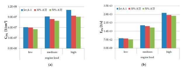
**Figure 8.** The number concentration  $C_{PN}$  (**a**) and intensity of the particles number emission  $E_{PN}$  (**b**) for tested fuels in three ranges of engine operation.
