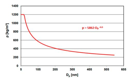
Figure 4. Density of solid particles depending on their diameter [32].
