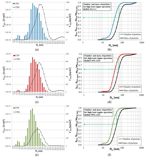
particles (Figure 7b) show that 90% of the relative number of all emitted particles is also 60% of their relative mass. About 90% of all particles is less than 70 nm in diameter.
