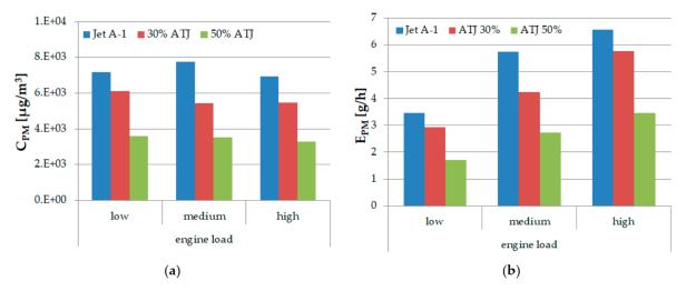
**Figure 9.** Mass concentration  $C_{PM}$  (**a**) and emission intensity of particulate matter  $E_{PM}$  (**b**) for tested fuels in three engine operation ranges.
