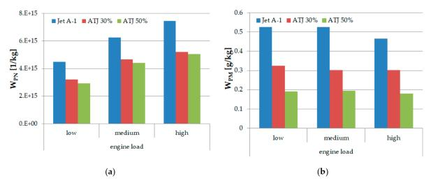
Figure 10. Particle number index  $W_{PN}$  (a) and particle mass index  $W_{PM}$  (b) for tested fuels in three engine load ranges.
