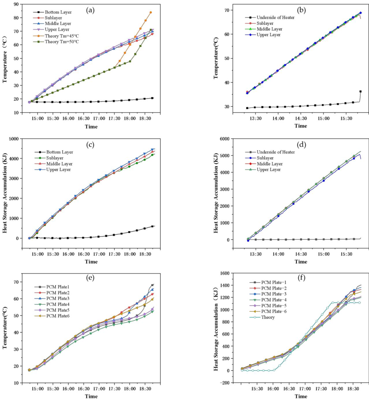
**Figure 6.** In working condition 1: (a) Water temperature curve of the PCM storage tank; (b) Water temperature curve of the common tank; (c) Heat storage accumulation curve of the PCM storage tank; (d) Heat storage accumulation curve of the common tank; (e) Temperature curve of the PCM plate; (f) Heat storage accumulation curve of the PCM plate.
