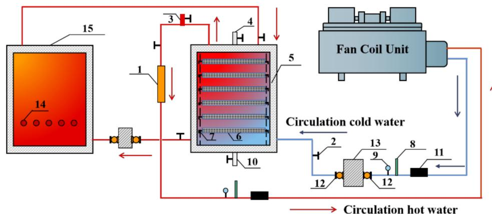
1-Glass rota meter; 2-Gate valve; 3-Exhaust three-way; 4-Filling pipe; 5-Insulating layer; 6-Phase change heat transfer plate; 7-Holder; 8-Precision thermometer; 9- Pressure meter; 10-outlet valve; 11-Platinum resistance; 12-Copper ball valve; 13-Pump; 14-Electrical heater; 15-Heating tank
