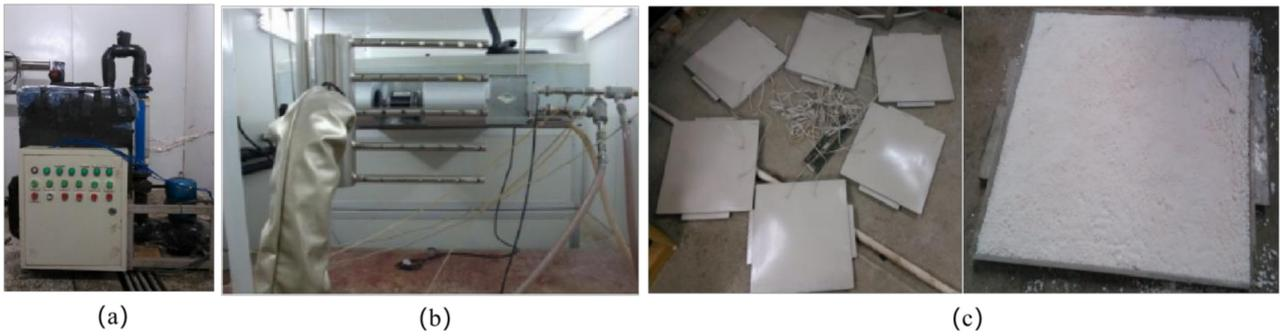
**Figure 4.** Main installations of the test-bed: (a) PCM storage tank; (b) Fan coil unit; (c) Phase change heat storage plates.
