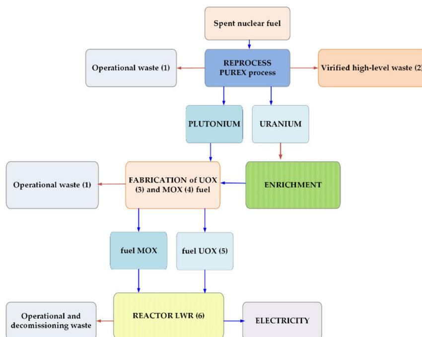
**Figure 7.** Reprocessing with reuse of uranium and plutonium. (1) Operational waste; (2) virified high-level waste; (3) uranium dioxide (UOX) fuel; (4) metal oxide (MOX) fuel; (5) fuel made of uranium dioxide; (6) light water reactor (LWR).
