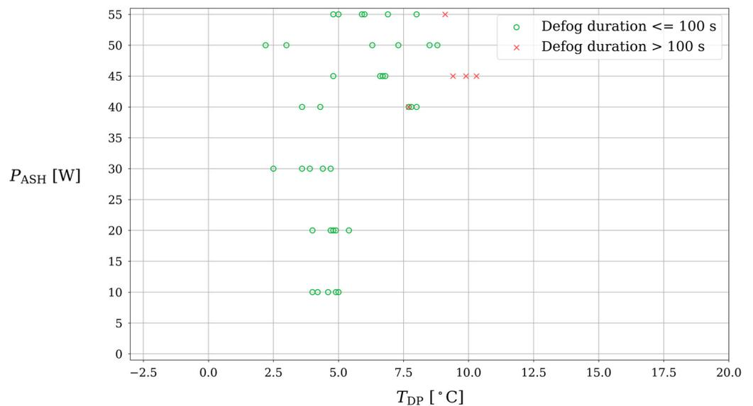
**Figure 2.** Measured correlation between a door-frame ASH's power usage and the DP.
