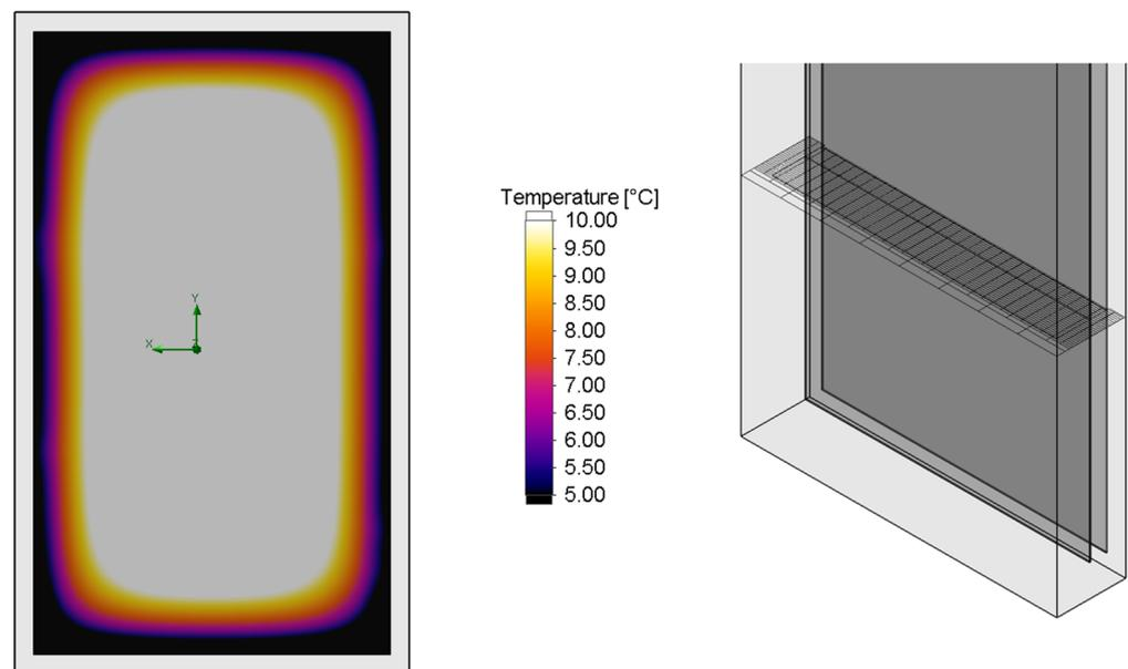
**Figure 1.** Simulation results for a 5W glass surface ASH. Inner glass surface temperature (**left**) and mesh granularity (**right**). The obstructing refrigerator body is hidden.
