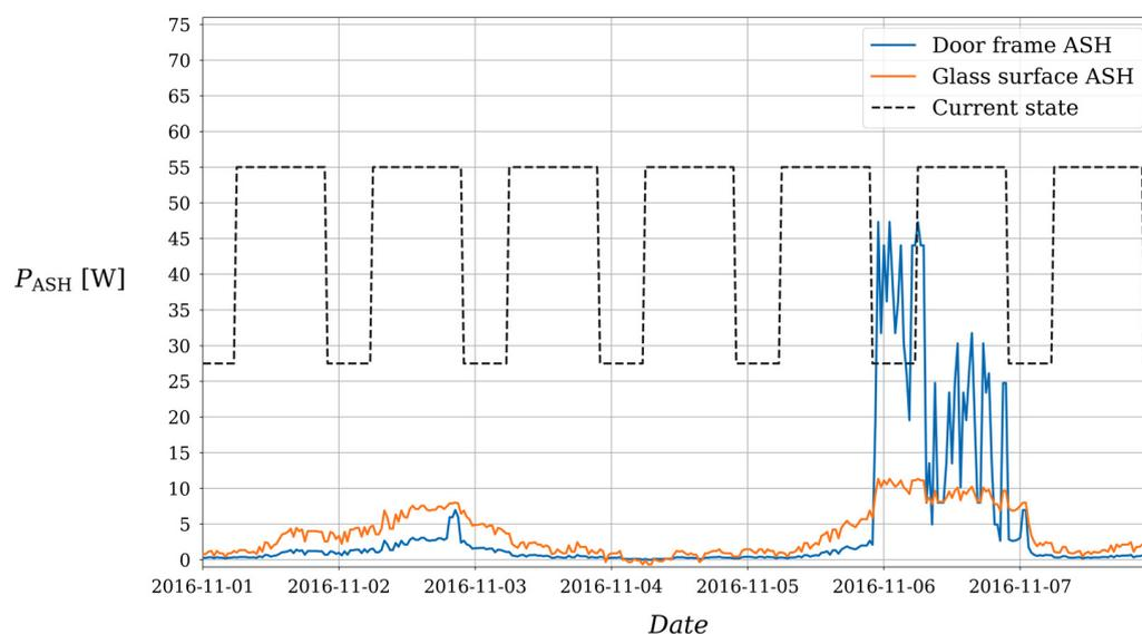
**Figure 6.** Optimal power usage according to the DP for both types of ASH.
