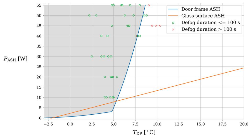
**Figure 3.** Comparison of the ASH's operating power vs the DP using a door-frame ASH and a glass ASH, with added measured data.
