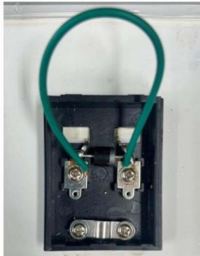
Figure 7. Diode short circuit.
