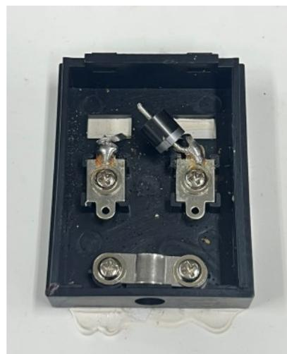
Figure 8. Diode open circuit.
