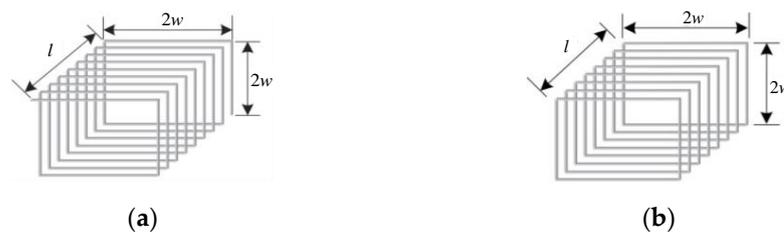
Figure 3. Schematic diagram of single layer square solenoid coil. (a) Real solenoid coil; (b) simplified solenoid coil model.
