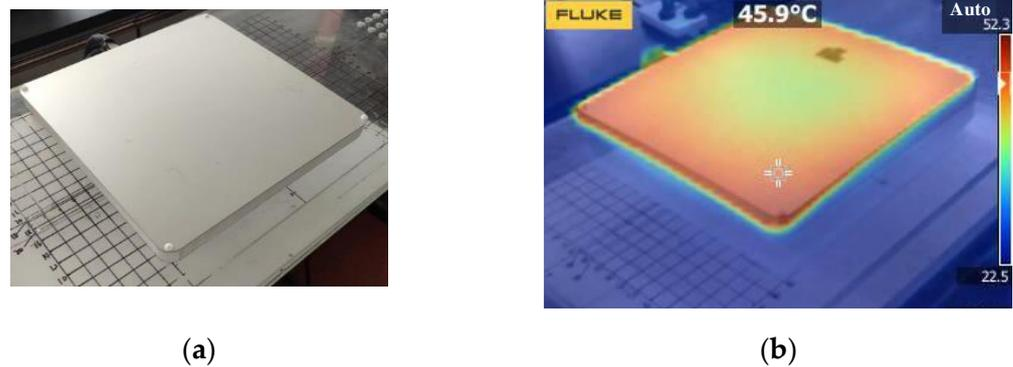
**Figure 22.** The temperature of the secondary shielding aluminum plate of the magnetic coupler. (a) The shielding aluminum plate; (b) the temperature value and distribution of the shielding aluminum plate.
