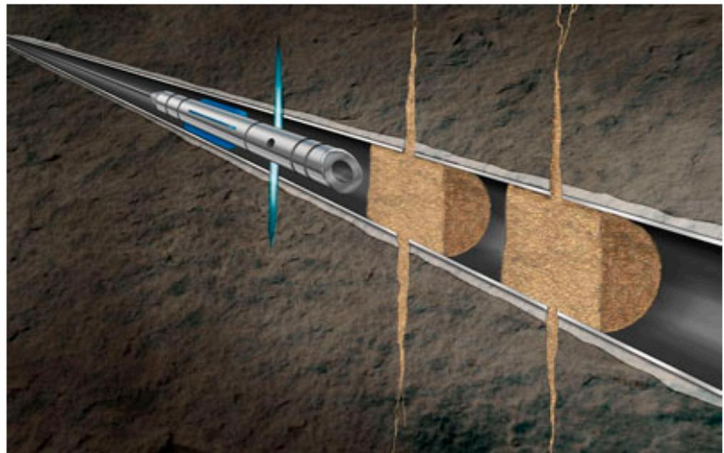
Figure 4. Schematic diagram of hydraulic jet fracturing.
