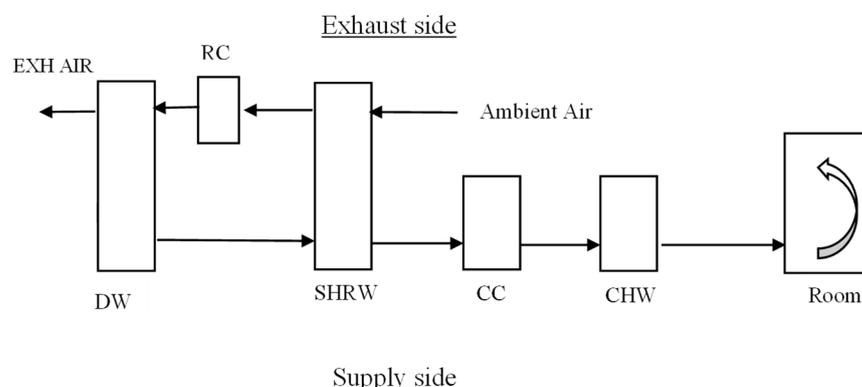
**Figure 1.** A proposed solid desiccant-based hybrid cooling system.
