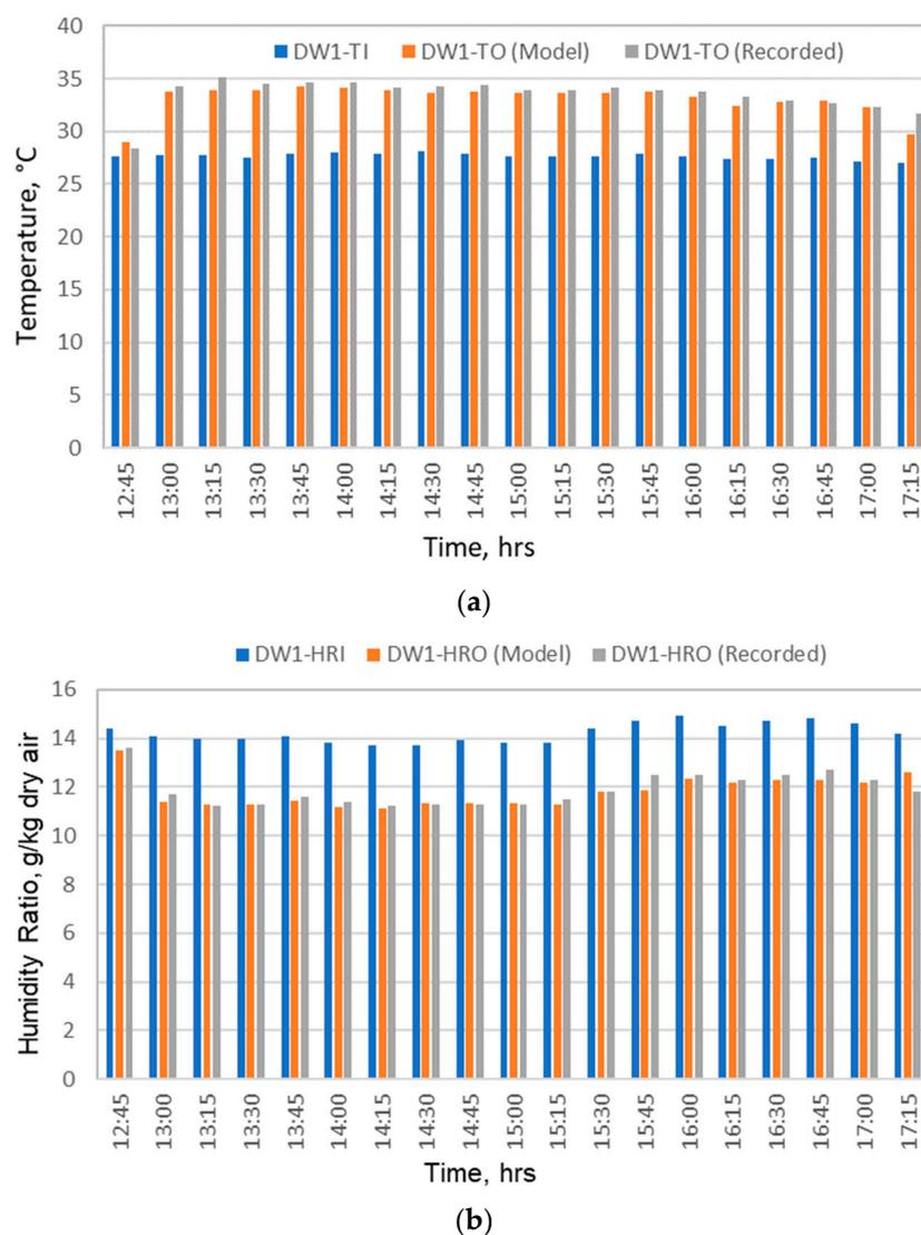
**Figure 4.** (a) Modelled and recorded values of (a) temperature across desiccant wheel (DW1) for day I, and (b) modelled and recorded values of humidity ratio across desiccant wheel (DW1) for day I.
