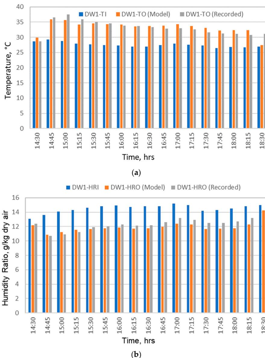
**Figure 5.** (a) Modelled and recorded values of temperature across DW1 for day II, and (b) modelled and recorded values of humidity ratio across DW1 for day II.
