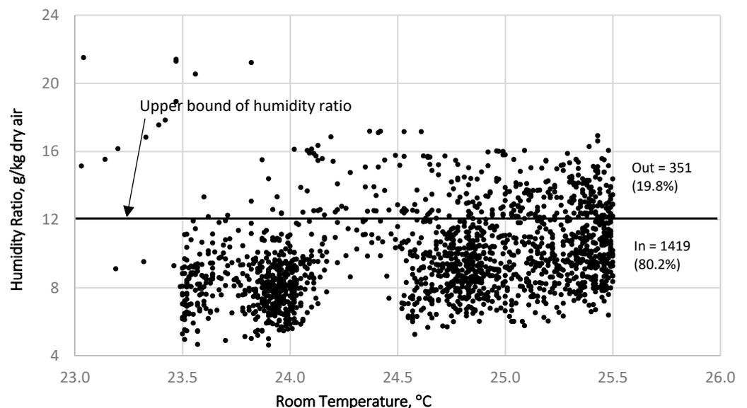
**Figure 7.** Plots of room temperature vs. humidity for Brisbane (system configuration with SHRW, regeneration temperature 90 °C).
