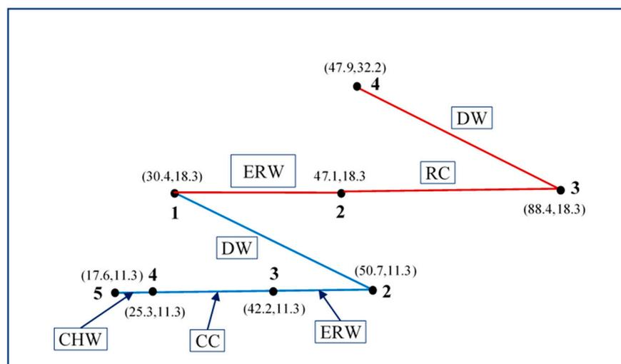
Figure 2. A typical psychrometric process of the proposed cooling system.
