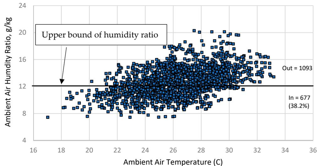
**Figure 6.** Plots of room temperature vs. humidity for Brisbane (Ambient condition).
