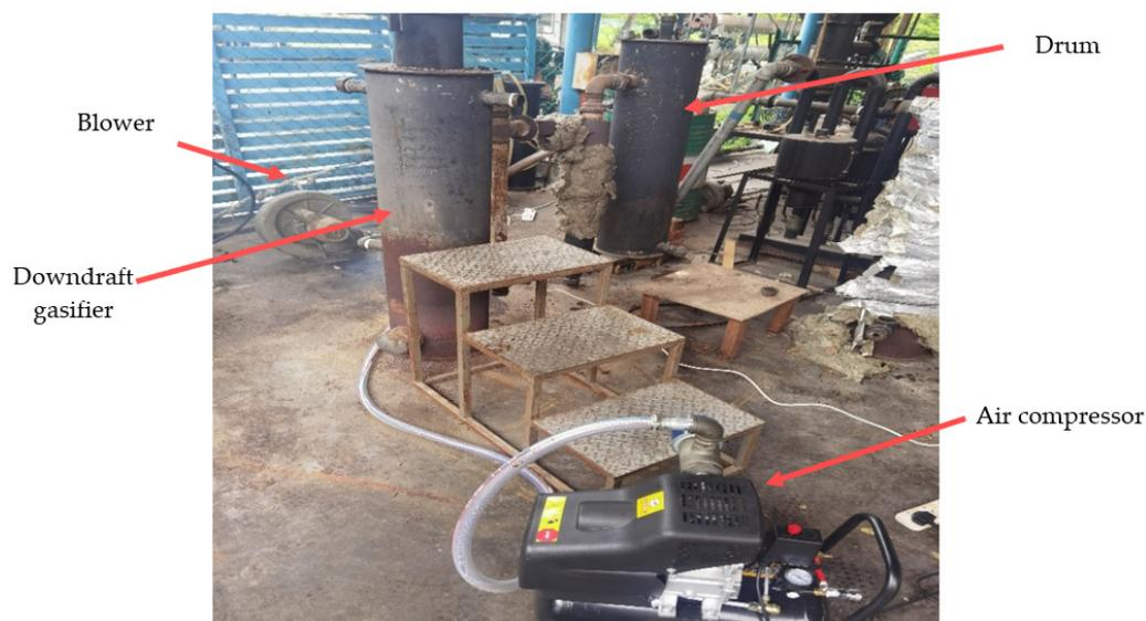
**Figure 2.** Setup of gasification.
