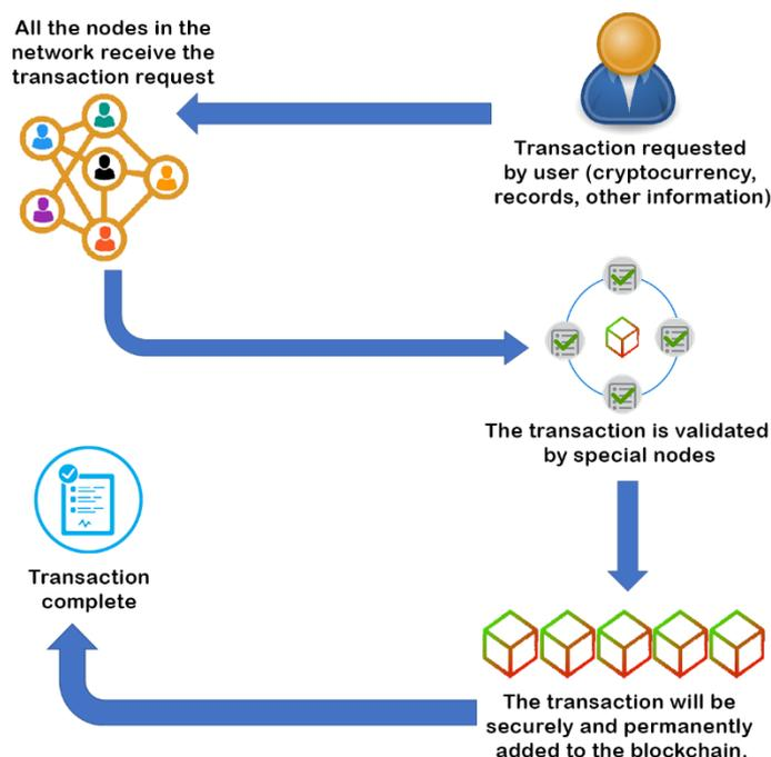
**Figure 5.** Transaction steps in the Blockchain network.
