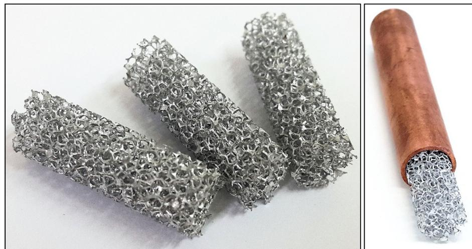
**Figure 1.** Cylinder-shaped metal foam elements applied in the experimental study.
