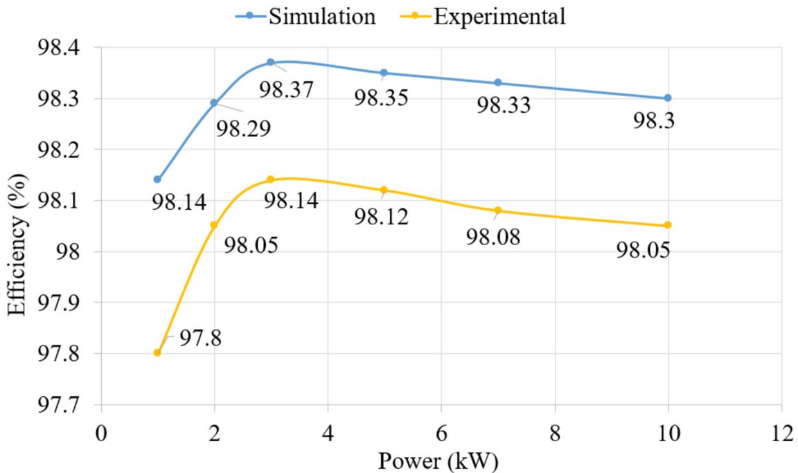
Figure 16. Efficiency as a function of the power: comparison between simulations and experimental results.
