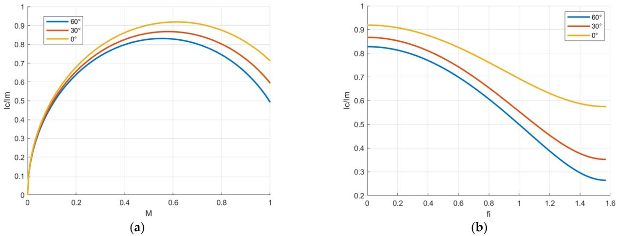
**Figure 6.** The rms DC-bus current normalized with respect to the peak of the phase current as a function of (a) the modulation depth  $M$ , and (b) the power factor  $\varphi$ , where the yellow line represents  $\delta = 0^\circ$ , the red line represents  $\delta = 30^\circ$ , and the blue line represents  $\delta = 60^\circ$ .
