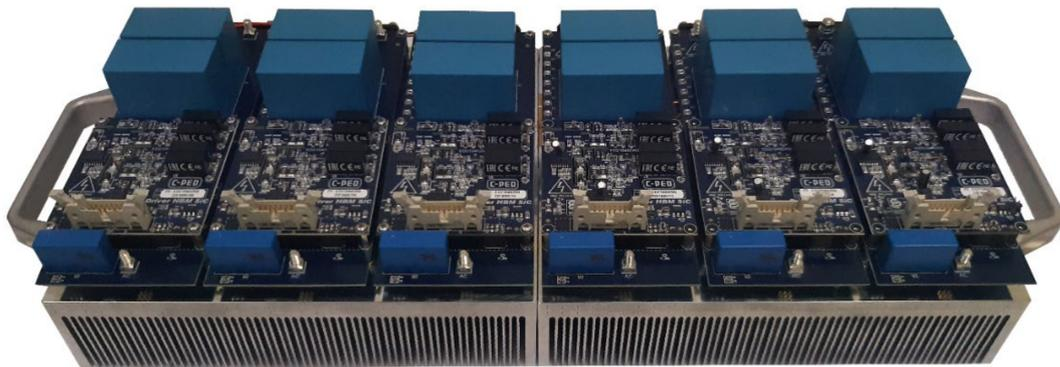
Figure 12. Prototype of the 6-phase boost rectifier.
