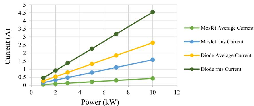
**Figure 2.** Average and rms current waveforms of the MOSFET and the diode as a function of the transfer power.
