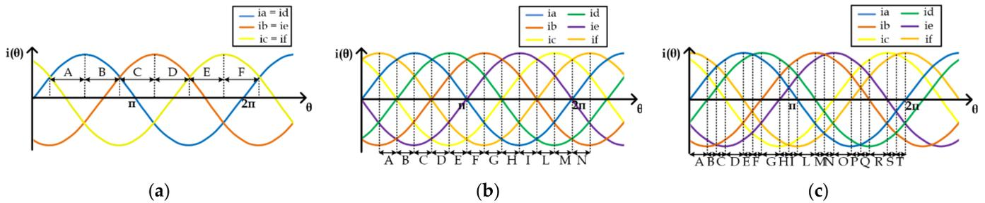
**Figure 4.** Phase current waveforms of the 6-phase boost rectifier considering (a)  $\delta = 0^\circ$ , (b)  $\delta = 60^\circ$ , and (c)  $\delta = 30^\circ$ .
