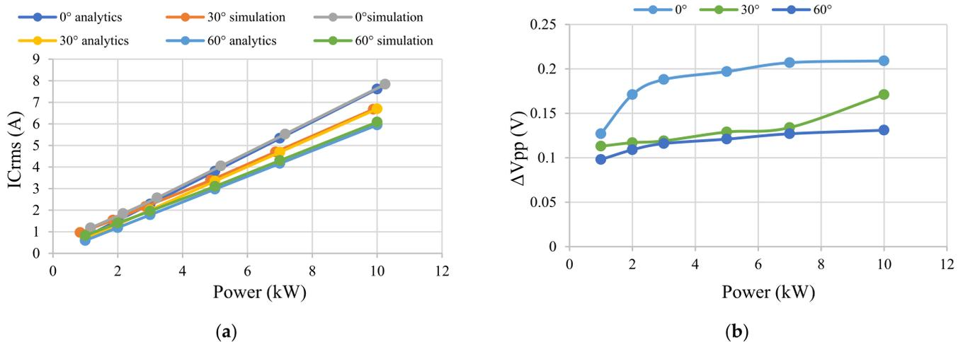
**Figure 11.** Simulation results of: (a) the DC-bus current stress, and (b) the voltage ripple.
