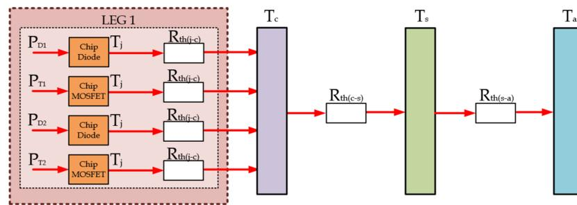
Figure 9. Equivalent thermal circuit.
