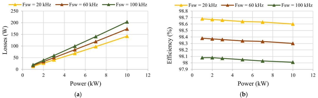
**Figure 3.** (a) Power losses  $P_{loss}$  of the 6-phase boost rectifier and (b) conversion efficiency assuming the switching frequency  $f_{sw}$  of 20 kHz (yellow line), 60 kHz (red line), and 100 kHz (green line), respectively.
