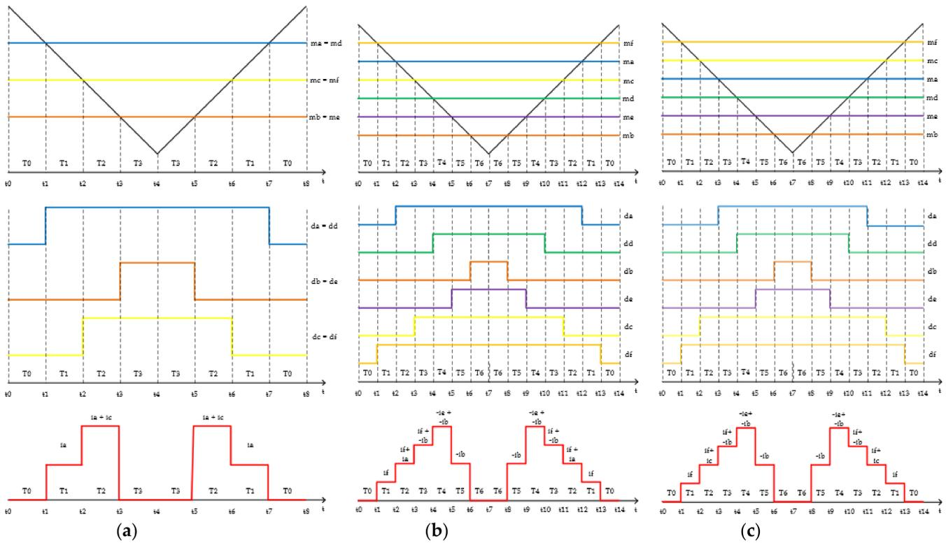
**Figure 5.** DC-bus current stress analysis in a switching period considering (a)  $\delta = 0^\circ$ ; (b)  $\delta = 60^\circ$ ; and (c)  $\delta = 30^\circ$ .
