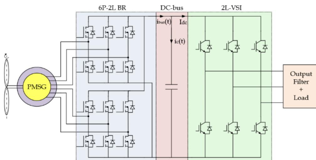
**Figure 1.** Power conversion system configuration.
