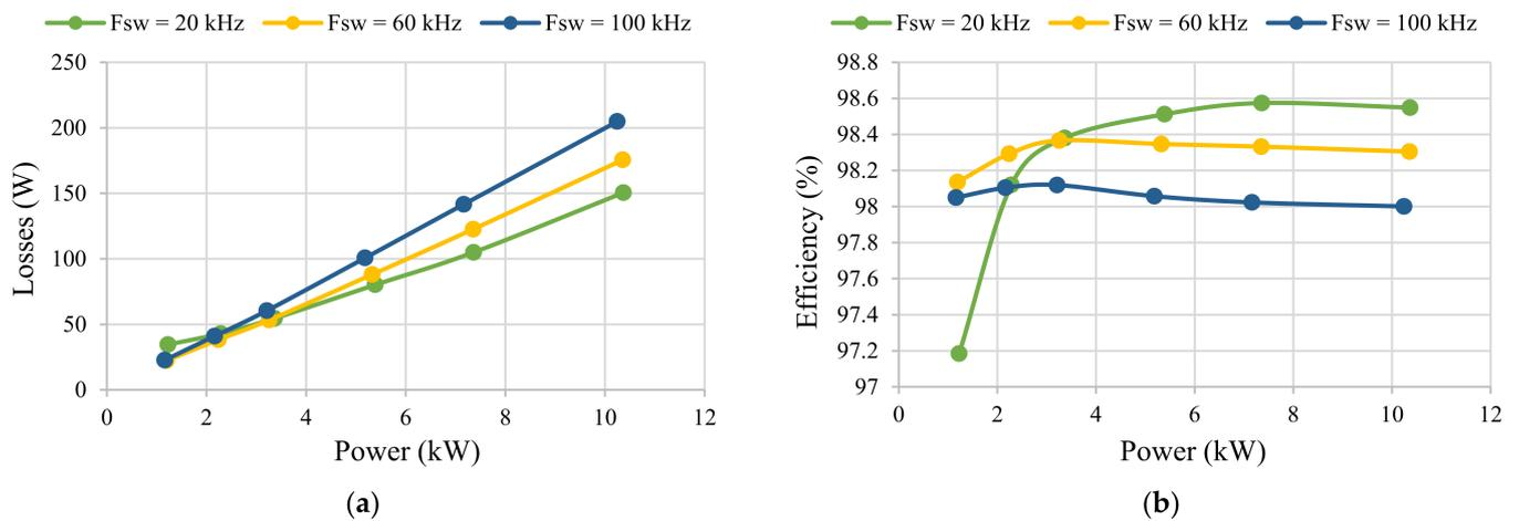
**Figure 10.** Simulation results of: (a) the power losses and (b) the power conversion efficiency assuming a switching frequency  $f_{sw}$  of 20 kHz (green line), 60 kHz (yellow line), and 100 kHz (blue line).
