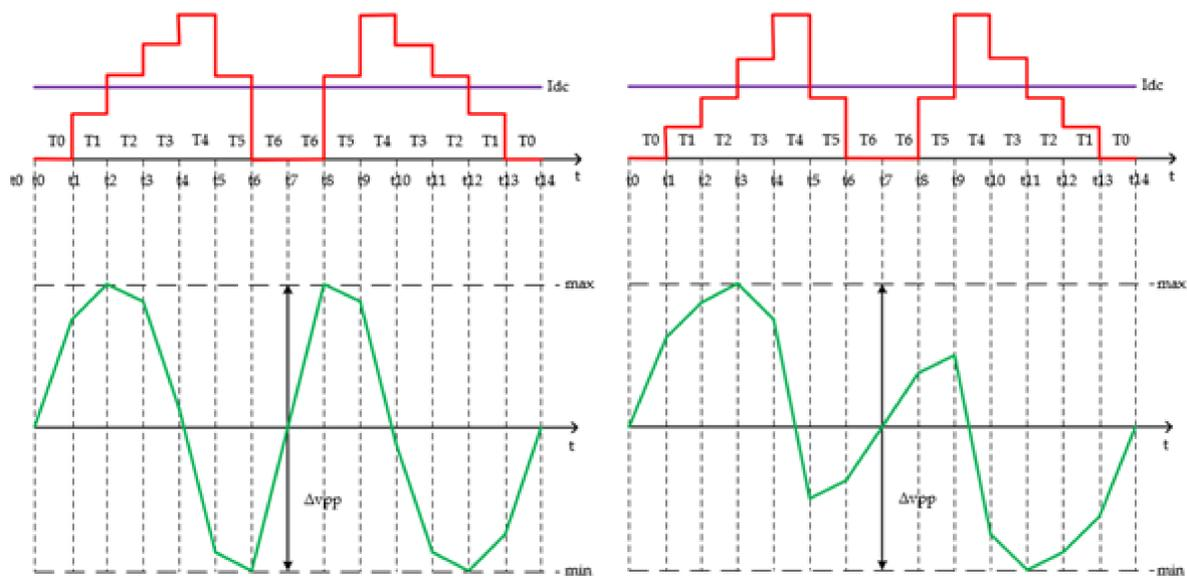
**Figure 8.** Voltage ripple analysis in the switching period considering  $\delta = 30^\circ$  and  $\delta = 60^\circ$ ,  $i_{bus}(t)$  (red trace),  $I_{dc}$  (violet trace), voltage ripple (green trace): (a) shows case A, in which  $I_{dc}$  is lower than the phase current  $i_a$ ; (b) shows case B, in which  $I_{dc}$  is greater than the phase current  $i_a$ .
