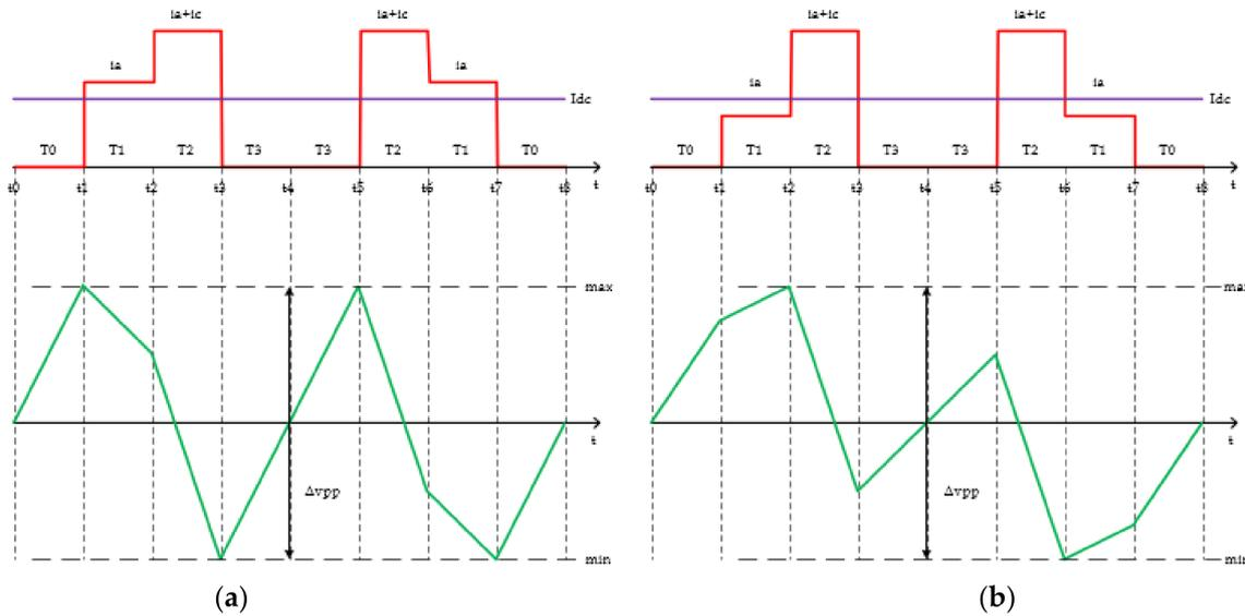
**Figure 7.** Voltage ripple analysis in the switching period considering  $\delta = 0^\circ$ ,  $i_{bus}(t)$  (red trace),  $I_{dc}$  (violet trace), and voltage ripple (green trace): (a) shows case A, in which  $I_{dc}$  is lower than the phase current  $i_a$ ; (b) shows case B, in which  $I_{dc}$  is greater than the phase current  $i_a$ .
