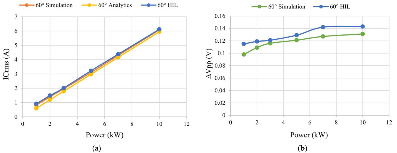
Figure 15. Comparison between HIL results, simulation results, and analytics results of: (a) the DC-bus rms current stress, and (b) the DC-bus voltage ripple power conversion efficiency assuming the phase displacement  $\delta = 60^\circ$ .
