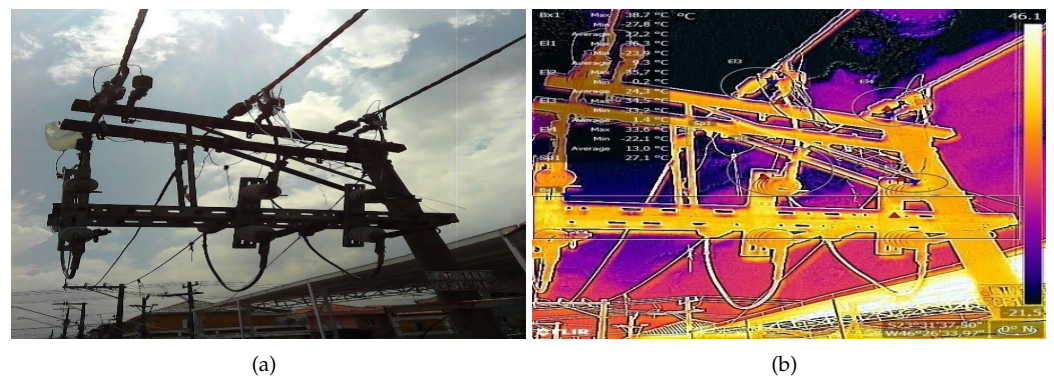
Figure 14. Outputs of using thermal cameras coupled in smartphones. (a) original images captured; (b) thermal images captured.
