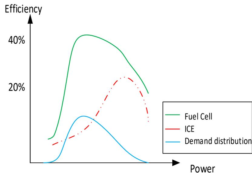
**Figure 7.** Fuel Cell & ICE Power Efficiency Curves [41].
