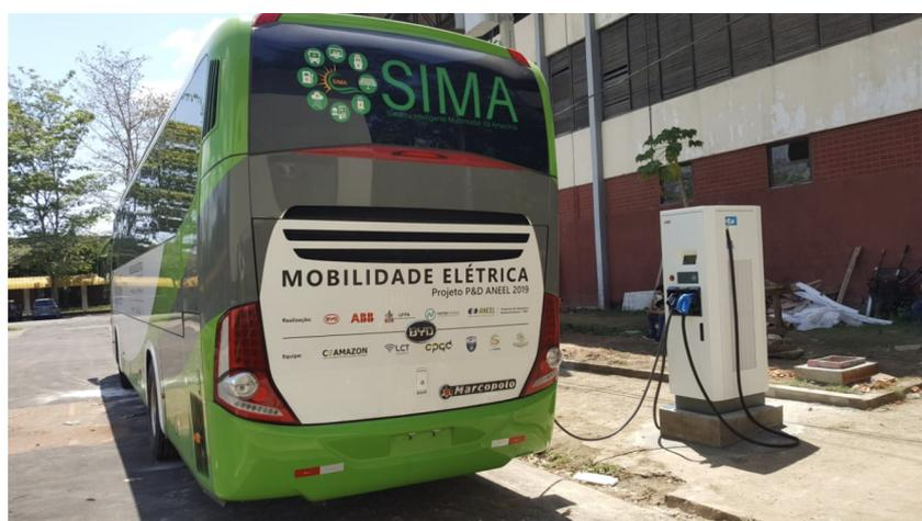
**Figure 6.** EV and charging station deployed at the main campus of UFPA.
