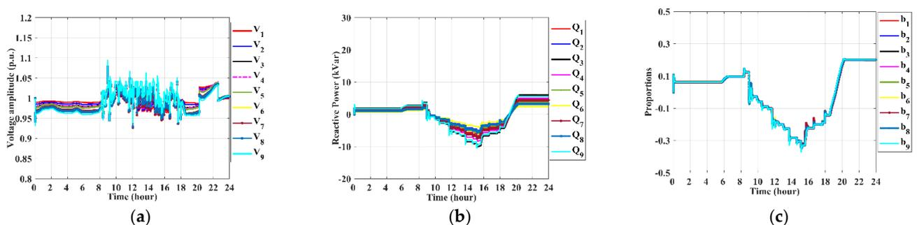
**Figure 7.** Node voltage fluctuation with OLTC and PV reactive power: (a) Nodal voltage fluctuation; (b) PV reactive power output; (c) proportions of reactive power.
