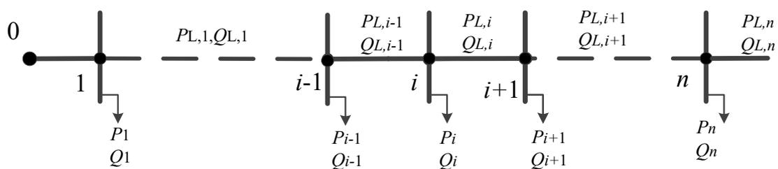
Figure 2. Network topology diagram of LVND.
