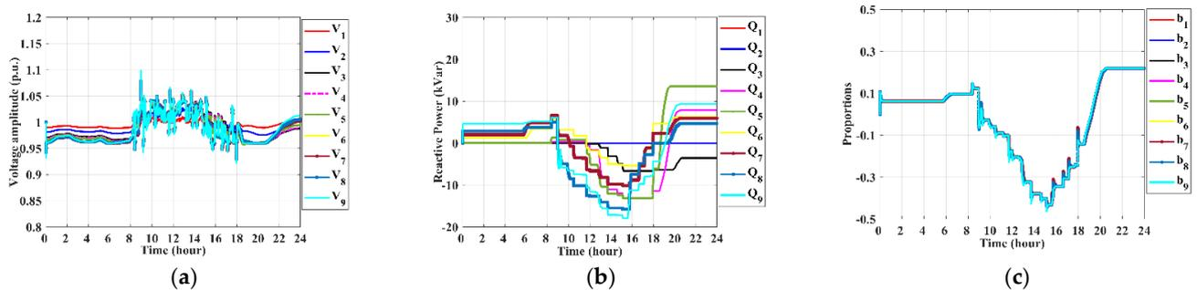
**Figure 6.** Nodal voltage magnitudes with reactive power sharing: (a) Nodal voltages; (b) reactive power of PV sources; (c) reactive power ratio of PV sources.
