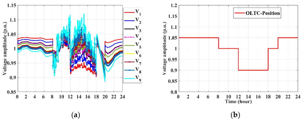
**Figure 8.** Node voltage fluctuation only with OLTC: (a) Nodal voltage fluctuation; (b) the tap position of OLTC.
