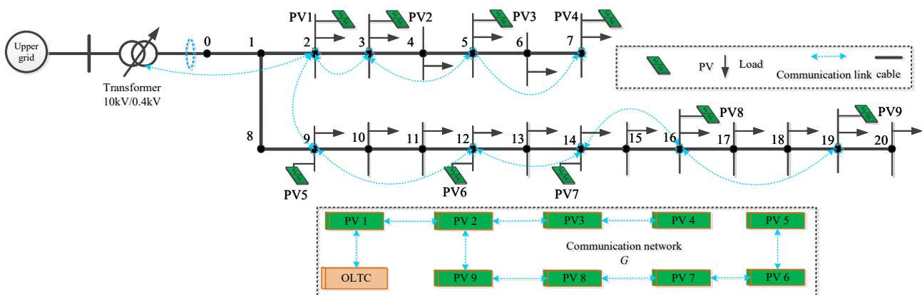
**Figure 1.** Node voltage regulation model of LVDN with a high proportion of distributed PV sources. The black arrow is the load of each node, while the dash blue lines with arrow are the communication links.
