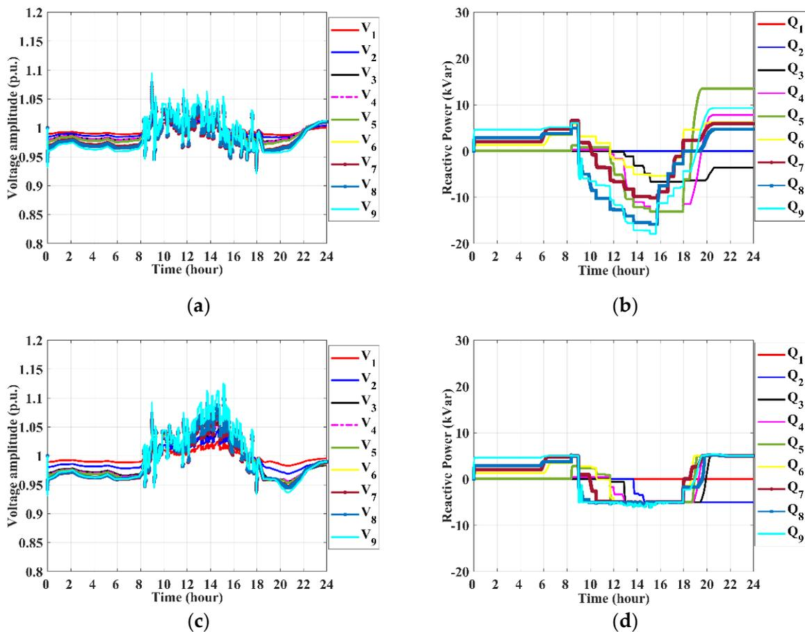
**Figure 5.** Voltage fluctuations: (a) Node voltage fluctuation; (b) photovoltaic reactive power output; (c) node voltage fluctuation with reactive power limits; (d) photovoltaic reactive power output with constraints.
