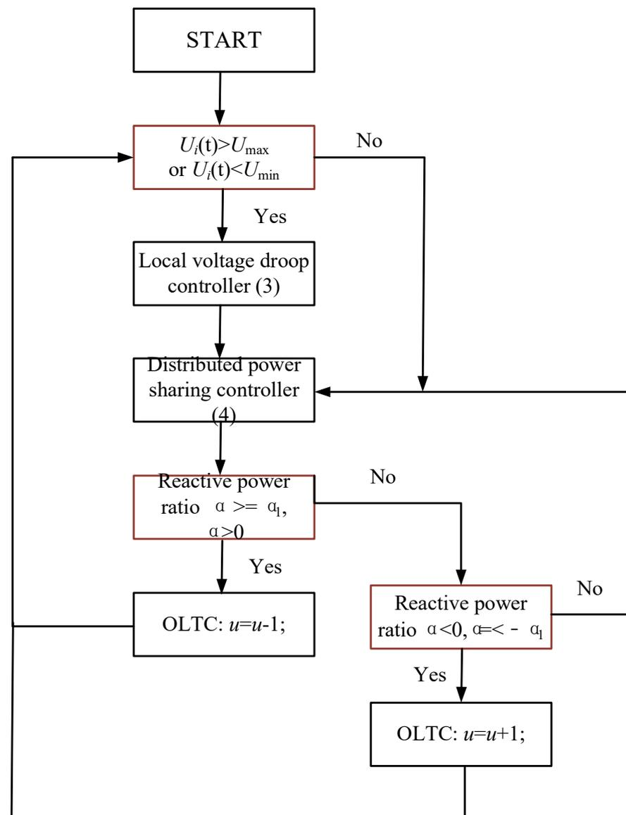
Figure 3. The flowchart of the proposed voltage regulation method.
