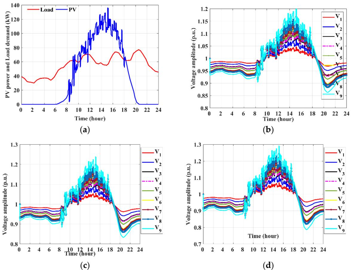
**Figure 4.** Node voltage fluctuation without regulation strategy: (a) Total PV power output and total load demand; (b) the fluctuation of node voltage amplitude; (c) the voltage amplitudes with 1.2 times the length of cables; (d) the voltage amplitudes with 1.5 times the length of cables.
