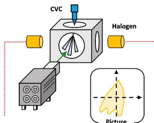
**Figure 3.** Schematic of fuel atomization tests using halogen lighting—longitudinal projection view of fuel spray.
