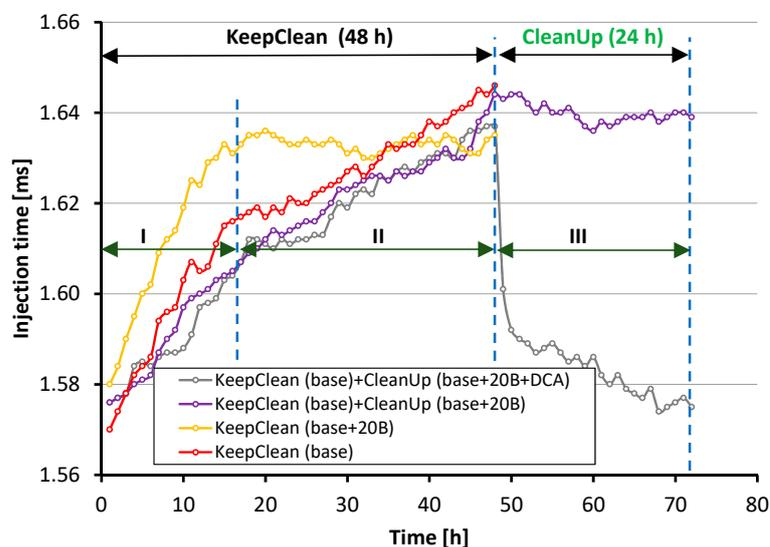
**Figure 6.** Changes in injection time of single doses of tested fuels obtained in Keep-Clean and Clean-Up tests.
