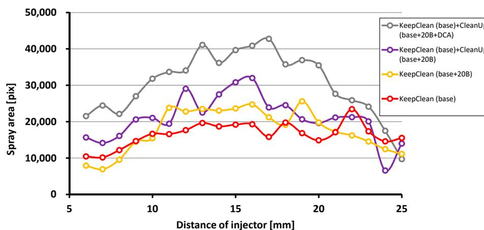
Figure 11. The course of changes in the areas of the fuel spray (the sum of the six streams from the beginning of the analysis—6 mm to the end—25 mm) in cross-sections.
