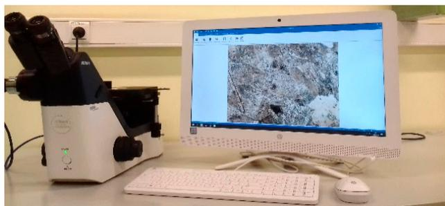
**Figure 5.** An upgraded Nikon Eclipse MA100N metallographic microscope used for visual observations of the nozzle tip of the GDI system injector under study.
