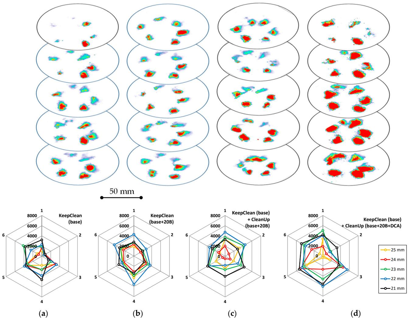
**Figure 10.** Cross-sectional view of the jet (a–d) and area analysis (below) of individual fuels after Keep-Clean and CleanUp tests: (a,b) tests lasting 48 h and (c,d) tests lasting a total of 72 h.
