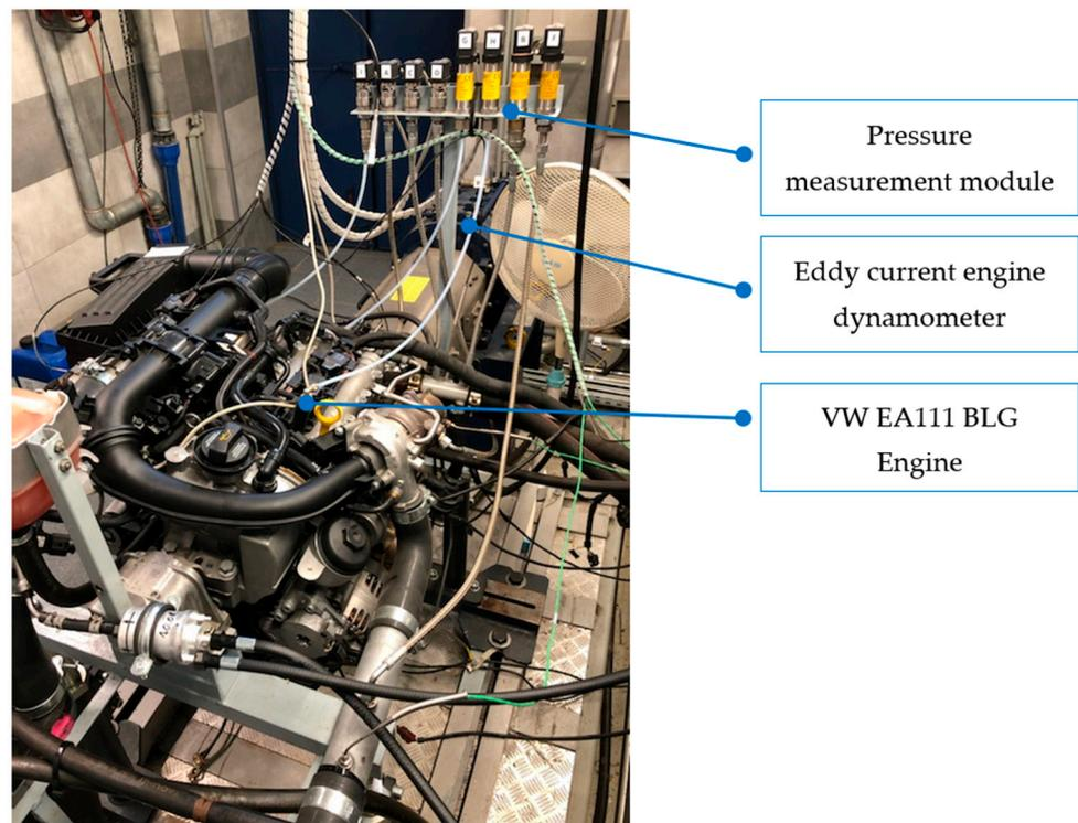
Figure 1. General view of test stand with VW EA111 BLG engine (photo INIG-PIB).
