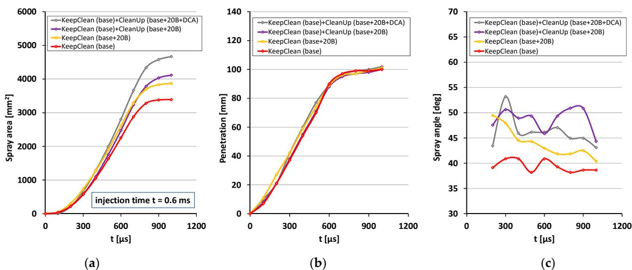
**Figure 8.** Analysis of geometric indices of the atomized fuel spray (six fuel jets were considered combined): (a) spray area; (b) penetration; and (c) jet cone angle.
