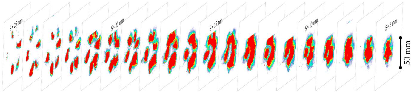
**Figure 9.** Sequence of images of the fuel jet in cross-section; the view includes the full sequence of tests from 6 to 25 mm from the tip of the atomizer.
