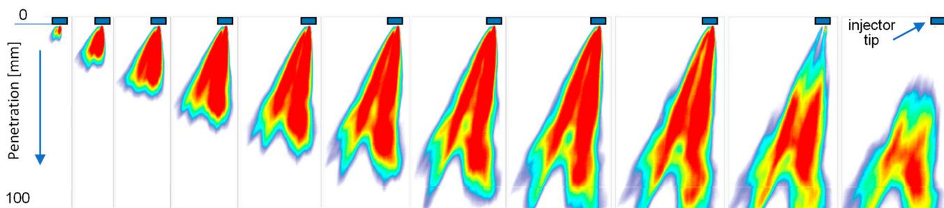
**Figure 7.** Sequence of fuel spray formation images filmed at 10 kHz ( $\Delta t = 100 \mu\text{s}$ ) in a constant volume chamber (example fuel spray pattern—maximum penetration  $S = 102 \text{ mm}$ ).
