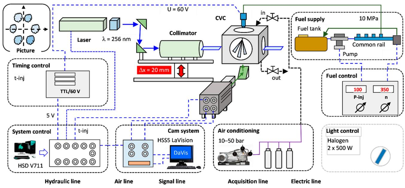
Figure 2. Schematic diagram of the structure of the fuel atomization test stand using laser illumination—cross-sectional views of all fuel jets.
