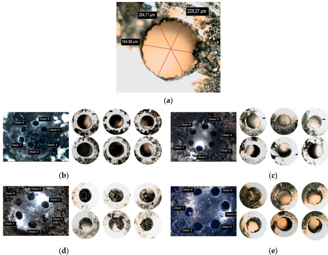
**Figure 12.** Images of the injector tips and holes after testing: (a) the hole diameter after the test as a determinant of the figure scale; (b) Keep-Clean (base); (c) Keep-Clean (base + 20B); (d) Keep-Clean (base) + CleanUp (base + 20B); and (e) Keep-Clean (base) + CleanUp (base + 20B + DCA).
