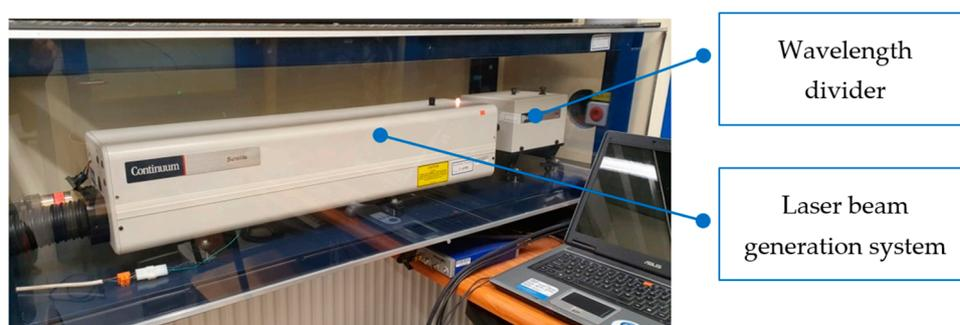
**Figure 4.** View of the laser beam generation system.
